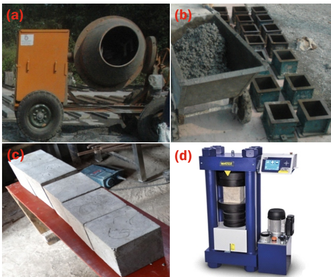
Fig.3: a) Motorized concrete mixer, b) Concrete moulds, c) Test specimen concrete cubes (15 X 15 X 15cm), d) Compressive strength testing unit.
