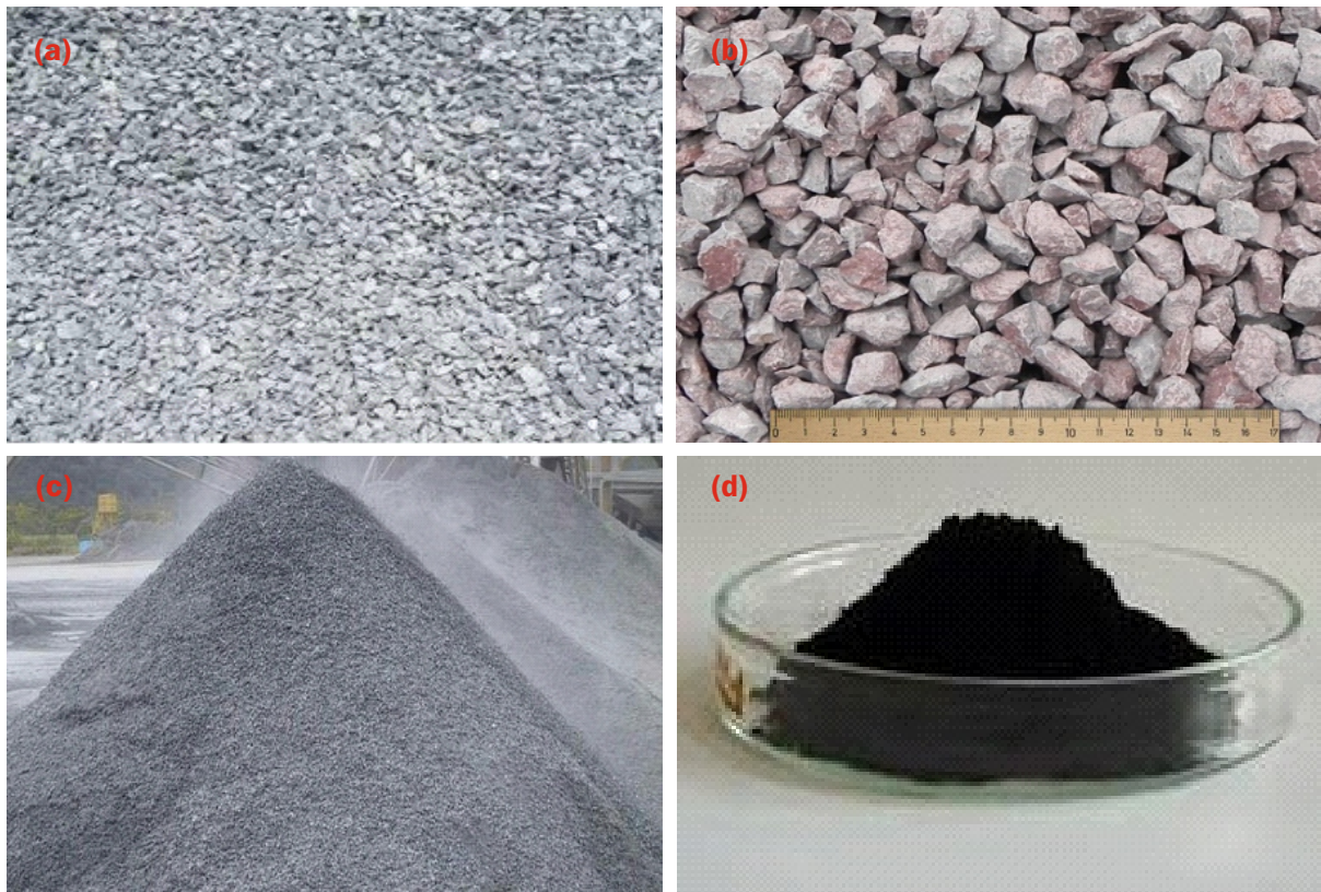
Fig.2: a) fine aggregate, b) coarse aggregate, c) crushed sand, and d) Graphene oxide used in preparation M30 concrete.
