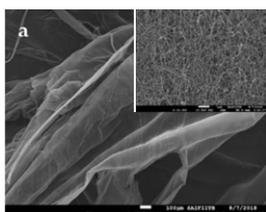
SEM image of Carbon nanotube wool. Inset a large network of isotropically oriented nanotubes
