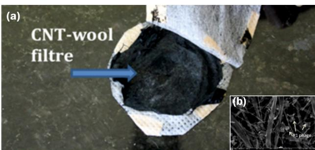
Fig.8: (a) Filter made from CNT wool (b) SEM image (inset) showing the P1 phage trapped in the filter.
