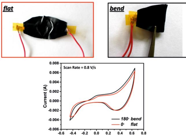
Fig.7: Variation of CV with bending of the flexible capacitor at a scan rate of 0.8 V/s.
