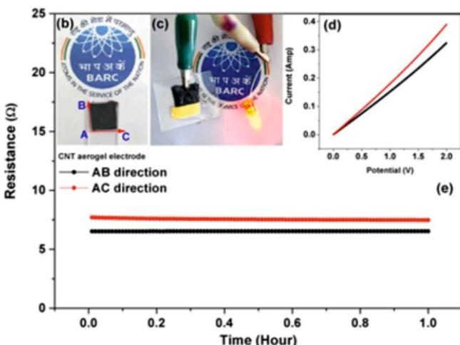
Fig.9: (a) Electrochemical impedance system for bio sensing and (b) CNT aerogel electrode (c) conductivity test (d) IV curve (e) chronoamperometry test of CNT aerogel electrode.
