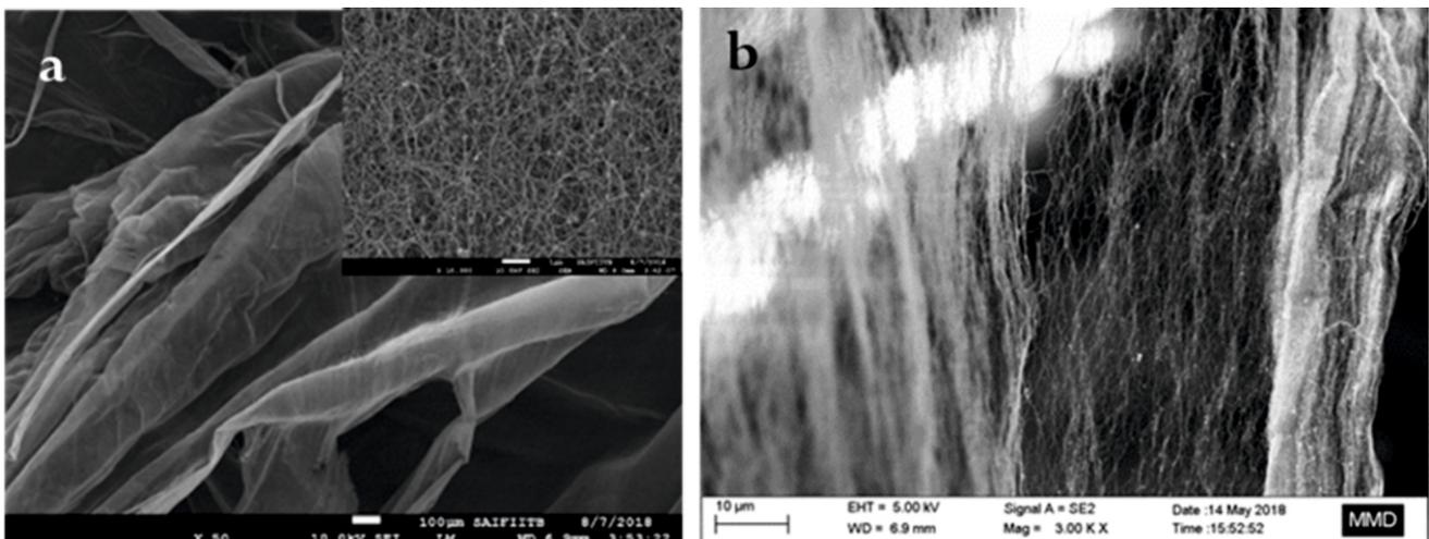
Fig.4: SEM images of (a) CNT wool and (b) CNT sheet.
