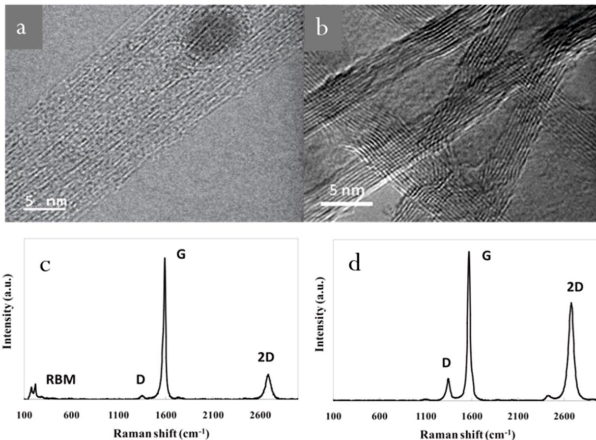
Fig.5: (a) TEM image of SWCNT bundles (b) TEM image of MWCNT (c) Raman spectrum of SWCNT (d) Raman spectra of MWCNT.
