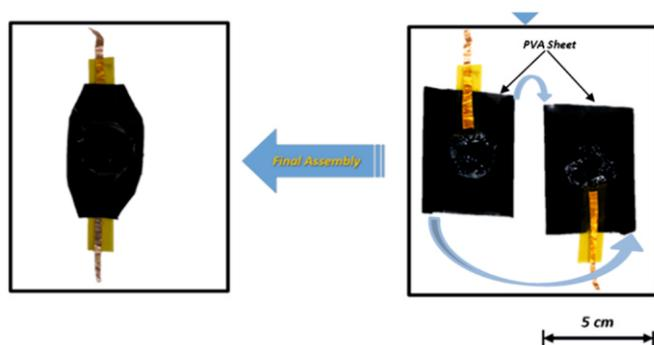
Fig.6: Preparation of a flexible capacitor.
