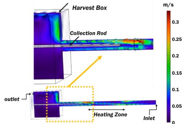
Fig.3: Velocity profile of the gas phase predicted by CFD.
