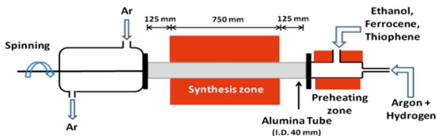
Fig.1: Schematic of the experimental setup for synthesis of CNT aerogel.
