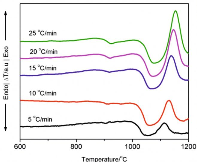
Fig.3: DTA plot of YAS glass powder at five different rates of heating.
