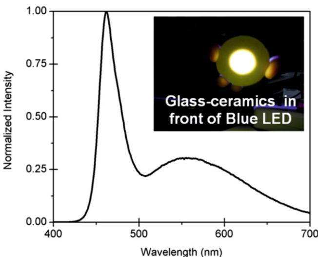
Fig.7: The illuminated glass-ceramics(inset) and the white light spectra as recorded by the PL spectrometer.
