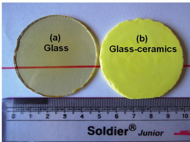
Fig.2: Polished YAS glass disk(a) and glass-ceramics phosphor(b).
