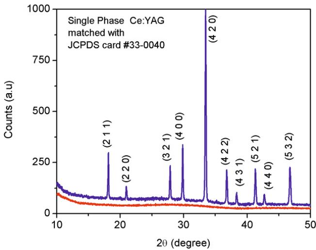
Fig.5: XRD pattern of as prepared YAS glass(red) and glass-ceramics phosphor(blue).
