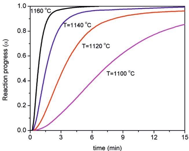
Fig.4: Isothermal predictions of the reaction progress(α) with time(min) at four temperatures (T °C).
