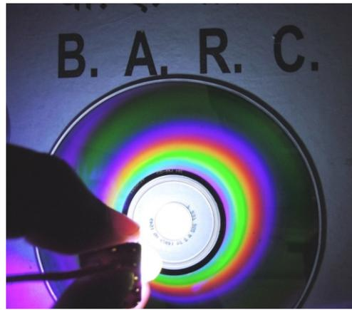
Fig.8: White light dispersed by a compact disk grating to create the rainbow.
