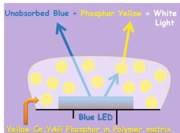
Fig.1: Schematic highlighting the working principle of white LED.
