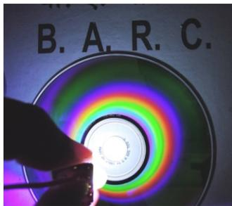
Demonstration of white light generation using Ce:YAG glass-ceramics phosphor
