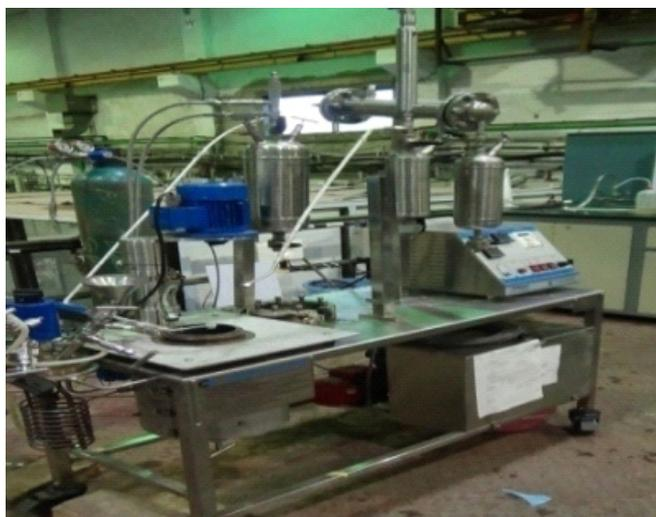
Fig.1: Autoclave for synthesis of PCS.
