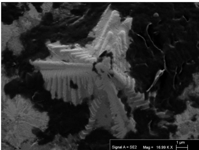
Fig.6: Micrograph of Ce:YAG dendrite at glass-ceramics surface.
