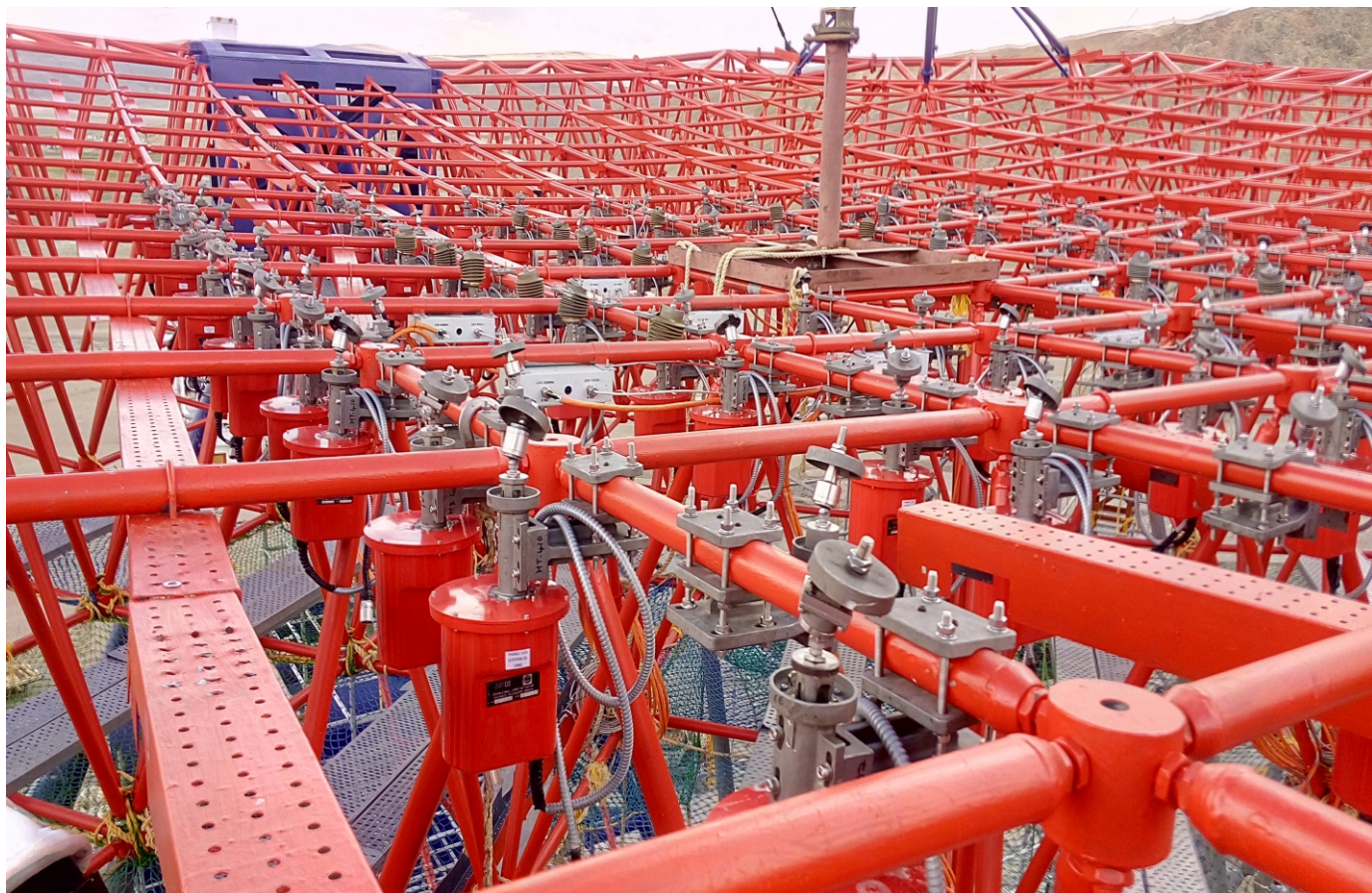
THE ACTIVE MIRROR ALIGNMENT CONTROL SYSTEM OF MACE is designed to realign all 356 mirror panels in an automated manner.
