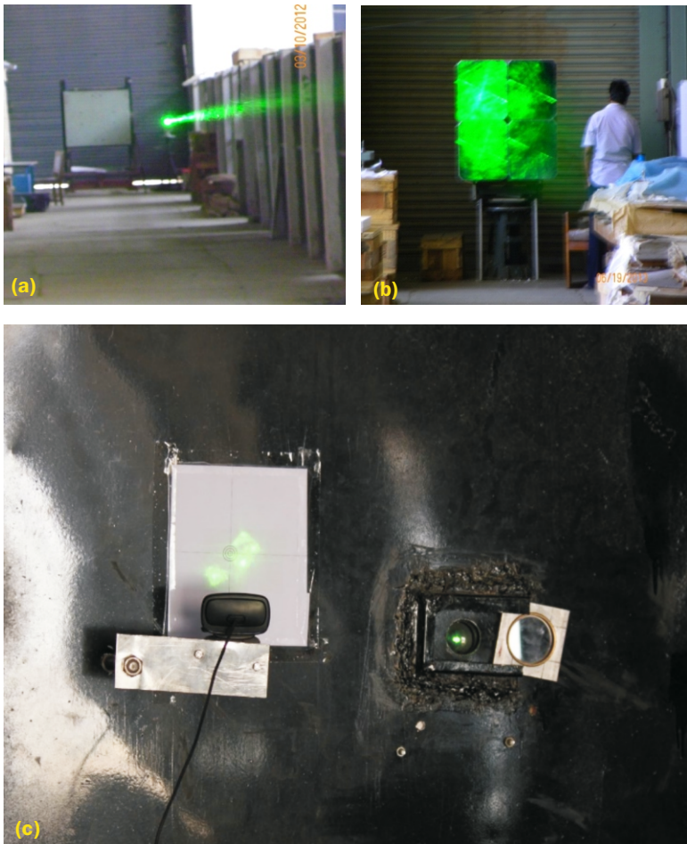
▲ TEST SETUP for alignment of mirror panel (a) Green laser with beam expander (b) 4 mirrors on a 1m x 1m panel (c) 4 unaligned spots due to 4 mirrors.
