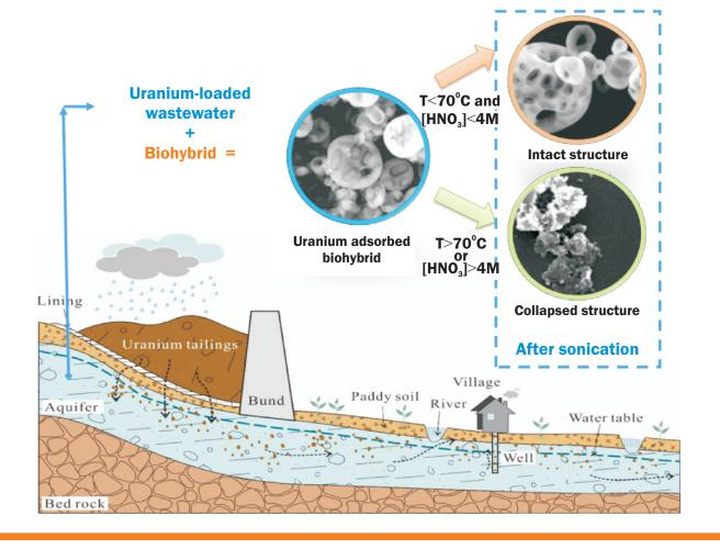
Release of adsorbed uranium from biohybrid adsorbents using ultrasound is established.
