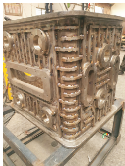
Fig.5: Separator shell with square bars as structural reinforcements and water flow channels.
