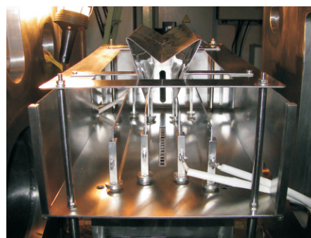
Fig.7: Assembly of electrostatic photo-ion collectors.
