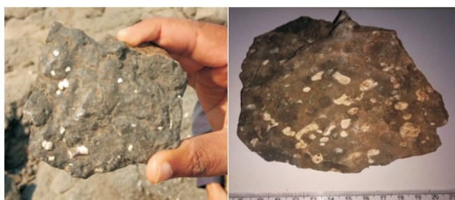
Fig.1: Naturally leached basalt glass collected from hot water springs located in Vajreshwari at Bhivandi Taluka of District Thane in Maharashtra State, India.
