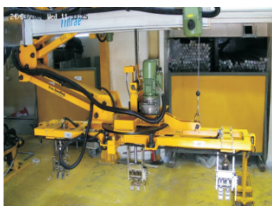
Cut-end Rod Handling System in operation
