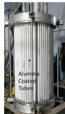
Fig.5: Alumina cooling tubes.
