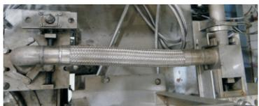
Fig.8: Three-Jaw connector & Block connector.
