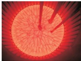
Molten glass pool inside Cold Crucible Induction Melter
