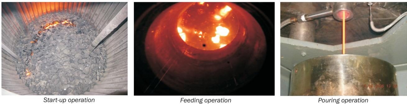
Fig.2: Different stages of industrial scale CCIM operation.
