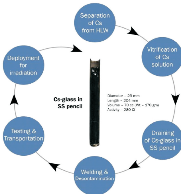
Fig.1: A thumbnail view of ^{137}\text{Cs} glass-pencil making process.
