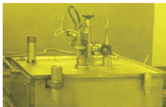
Fig.6: Welding of Cs glass pencil.
