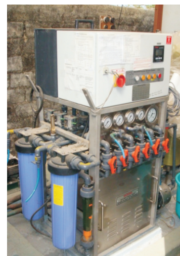
Fig.7: Disc Tube RO Pilot Plant.
