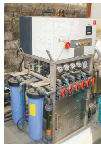
Fig.7: Disc Tube RO Pilot Plant.
