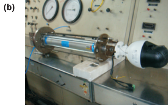
Fig.8: (a) Retractable Camera System for EP, (b) Retractable System with IP camera.
