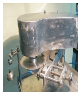
Fig.16: Remote cutting machine for disused sources.
