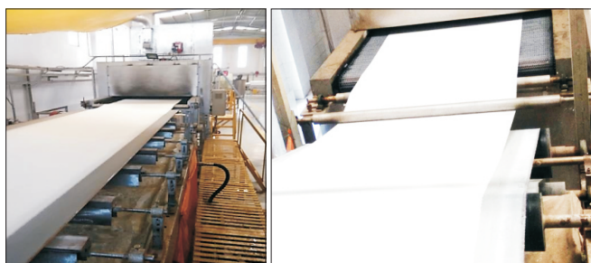
Fig.3: Mill scale of filter media manufacturing
