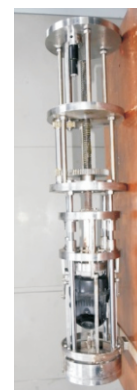
Fig.13: EP Hot-cell Retractable camera.
