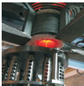
Fig.5: Pouring of Cs glass.
