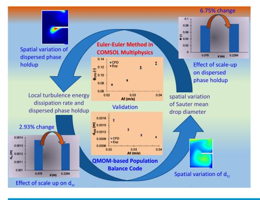
Coupled CFD-PB modelling is used to estimate dispersed phase holdup and Sauter mean drop diameter for liquid-liquid two-phase flow in a pulsed disc and doughnut column\*.
