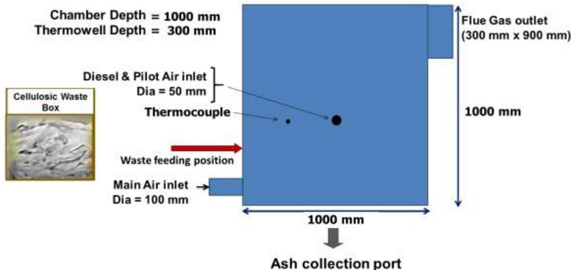
Fig.1: Schematic of primary chamber of incinerator setup
