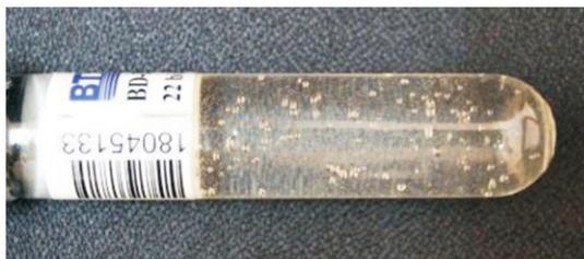
Fig. 8: Neutron generated bubbles in a bubble detector from deuterium target in D-D mode
