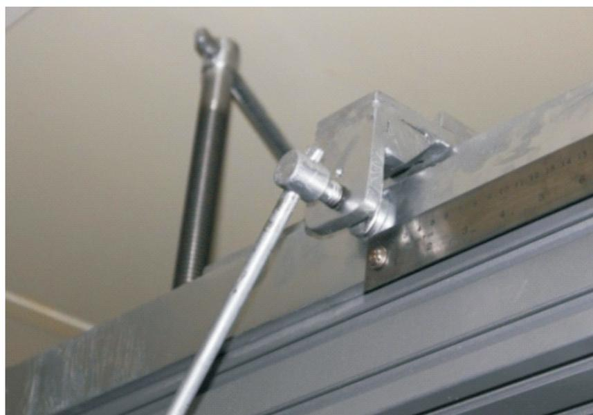
**Fig.3. Lock of X' axis of X-X' Table**
