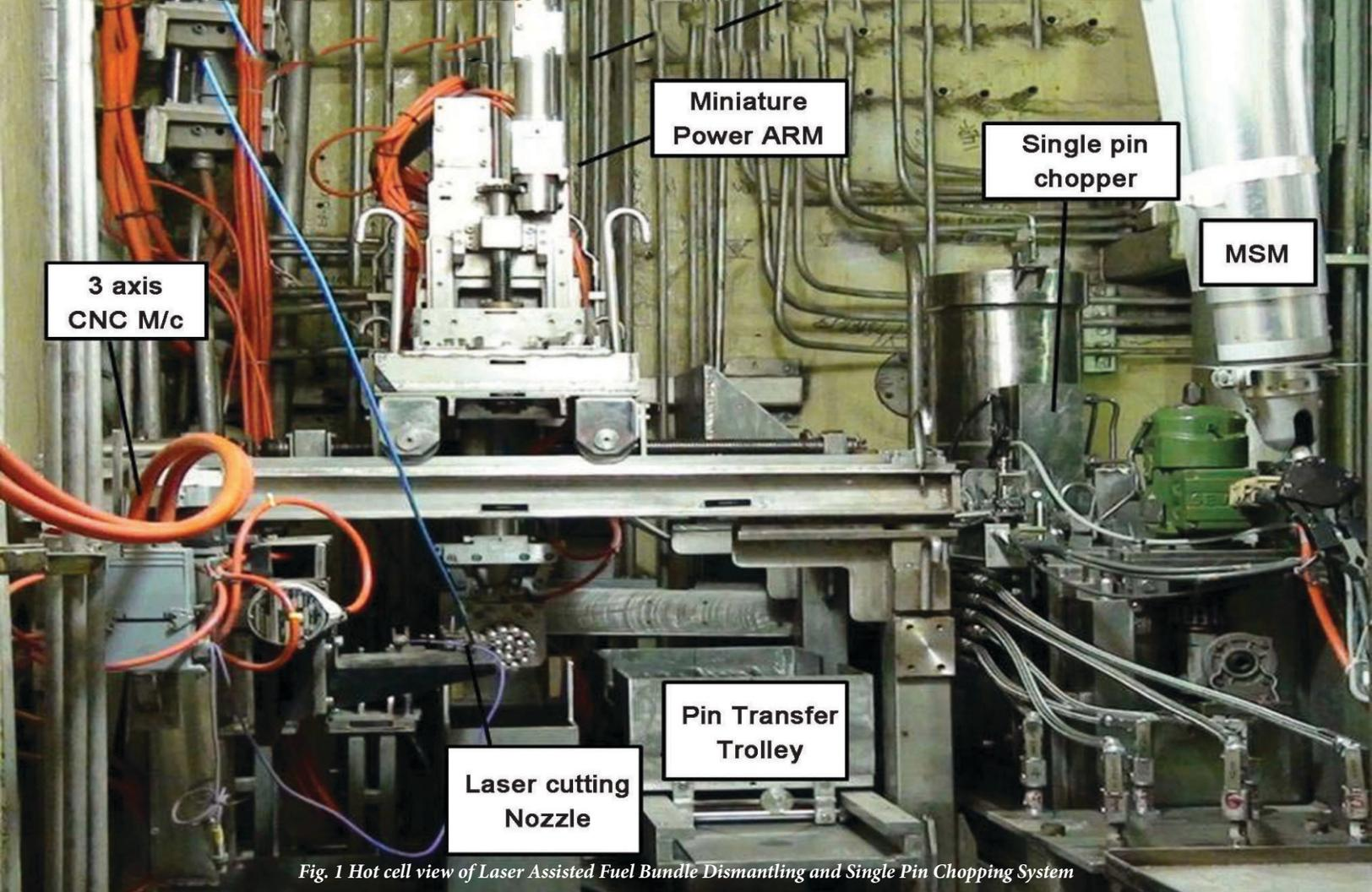
Fig. 1 Hot cell view of Laser Assisted Fuel Bundle Dismantling and Single Pin Chopping System
