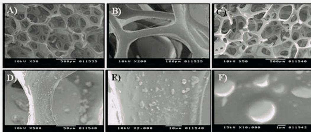
Fig. 2: SEM images: A-B) unmodified sponge with different magnifications. C-F) modified sponge with different magnifications showing rough surface consisting of micron, submicron and nano size hemisphere or bumps (ups and downs).
