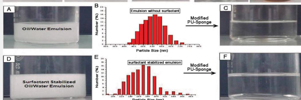
Fig.4: A-C) Photographs of emulsions without surfactant: before and after separation. D-F) with surfactant: before and after separation.
