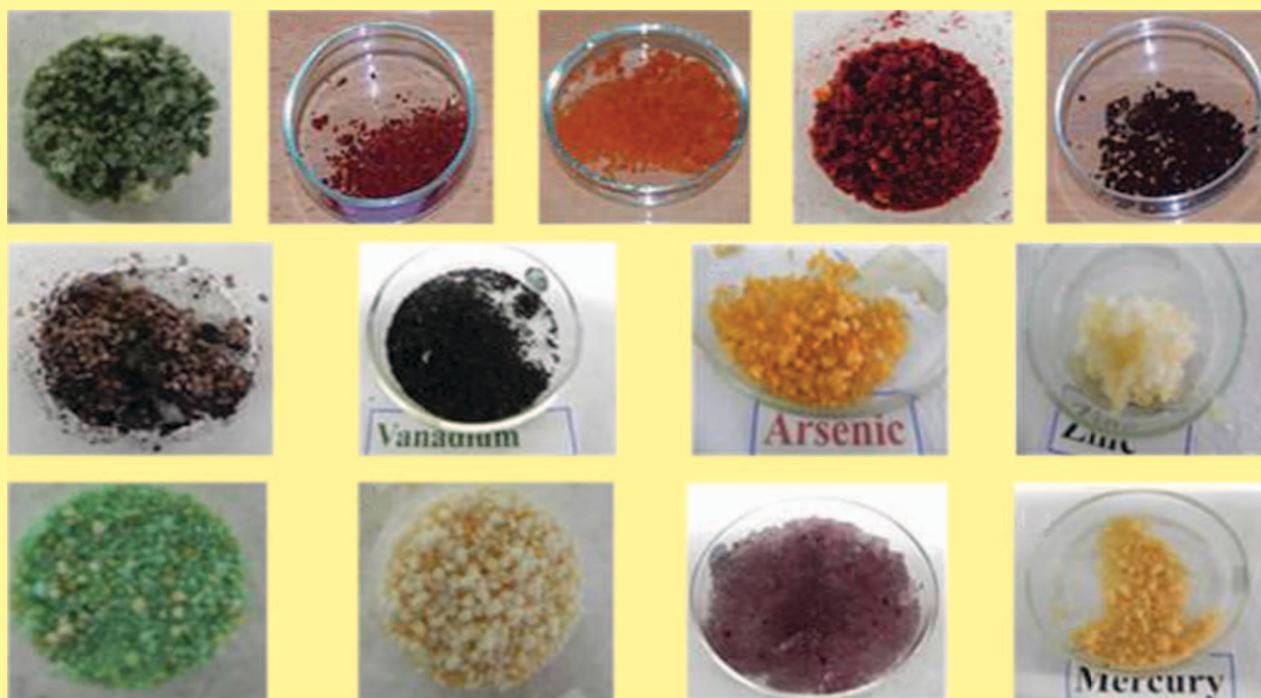
Metal sequestered complex of (A) PAH-Cr(VI) (B) PAH-Fe(II) (C) PAH- $UO_2^{*2}(VI)$ , (D) PAH-Fe(III) red mud with  $UO_2^{*2}(VI)$ , (E) PAH-Fe(II) with Fe(II) of ammonium ferrous sulphate, (F) PAH-Fe(II) with  $UO_2^{*2}(VI)$  and Cr(VI) (simulated solution) and others (vanadium-G, Arsenic-H, copper-I, Zinc-J, nickel-K, cadmium-L, manganese (M) and mercury (N))
