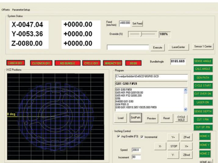
Fig. 3 GUI of CNC Machine
