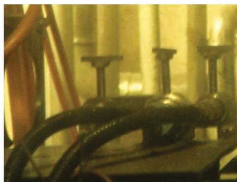
Fig. 6: Specially designed clamps for laser head and proximity sensors
