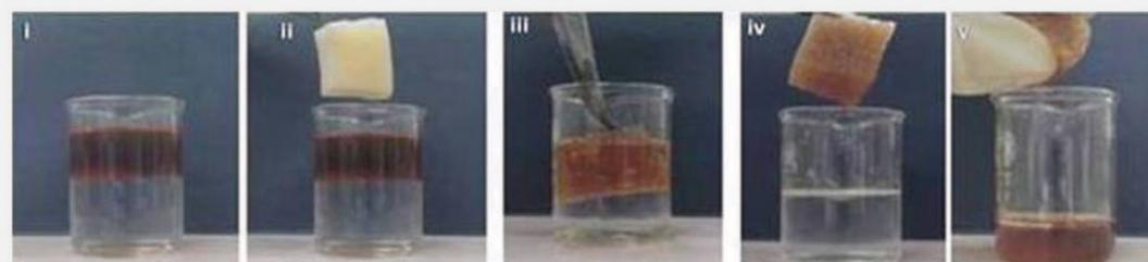
Fig.3: Diagrammatic representation of successive steps (i-v) of separating oil/water mixture and recollection of oil from it.
