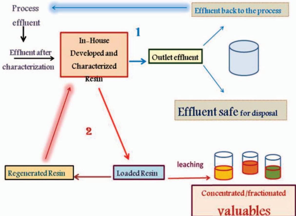
A schematic diagram of treatment of lean valuables bearing effluent
