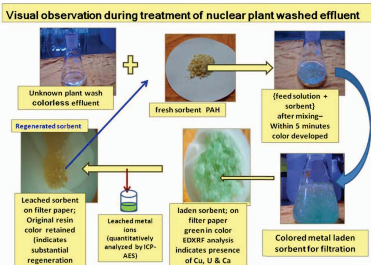
**Fig.4: A schematic methodology for the treatment of unknown effluents**
