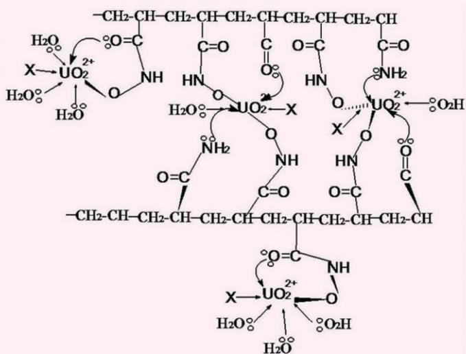
Fig. 5: Sequestration/Chelation of uranyl ions with PAH resin
