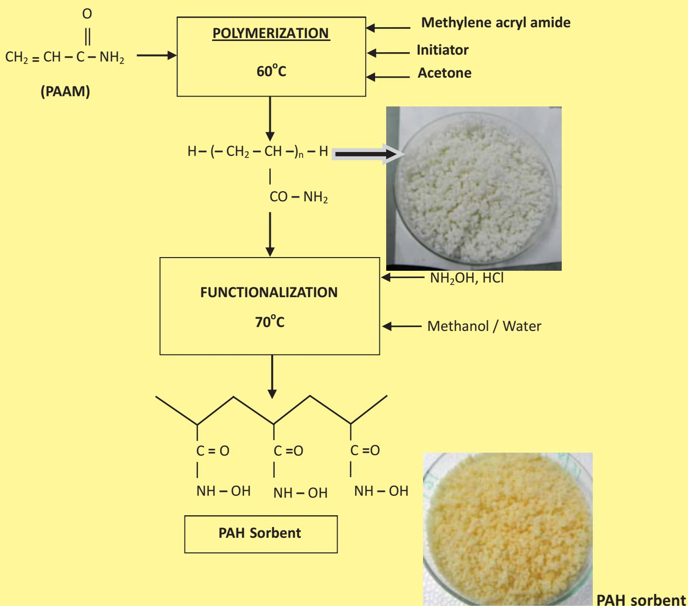
Fig.1: A schematic diagram of the preparation methodology of PAH sorbent
