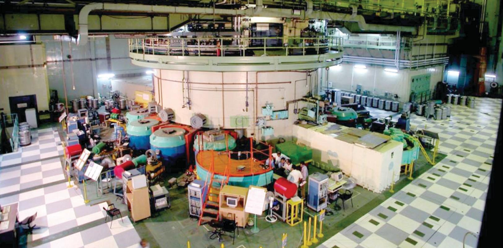
Dhruva is a research reactor, fuelled with metallic natural uranium. The reactor attained first criticality on August 8, 1985. The reactor caters to needs of broad spectrum multidisciplinary research and for production of various radioisotopes. Rated power of the reactor is 100 MW (thermal).
