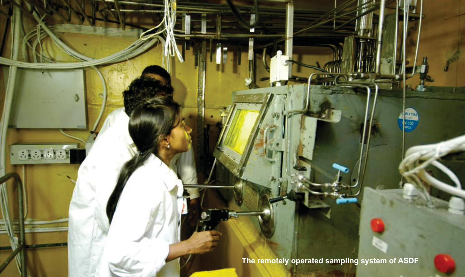
The remotely operated sampling system of ASDF
