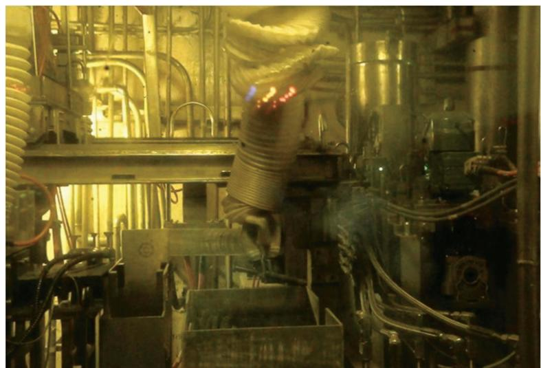
*Fig.11: Loading of fuel pin into the chopper using MSM*
