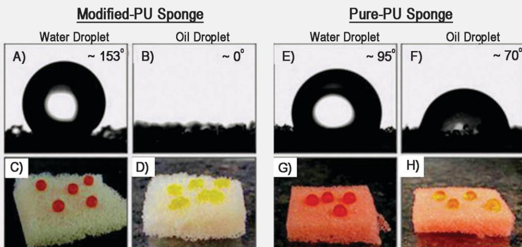
Fig.1: A-H) Images of contact angles (A-B, E-F) and beading (C-D, G-H) of liquid water (A,C,E,G) and oil (B,D,F,H) droplets on both the pure-PU sponge (E-H) and DMA-grafted PU Sponge (A-D).
