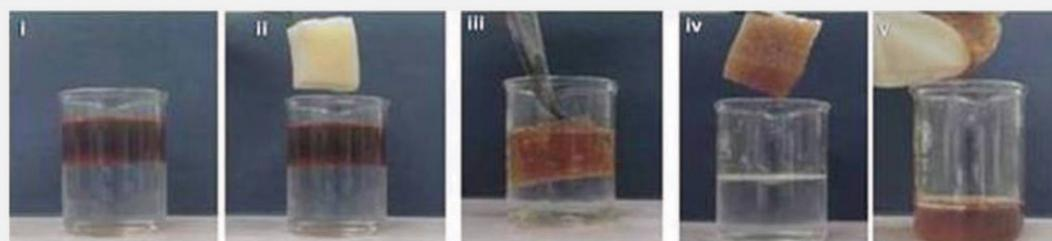
Fig.3: Diagrammatic representation of successive steps (i-v) of separating oil/water mixture and recollection of oil from it.
