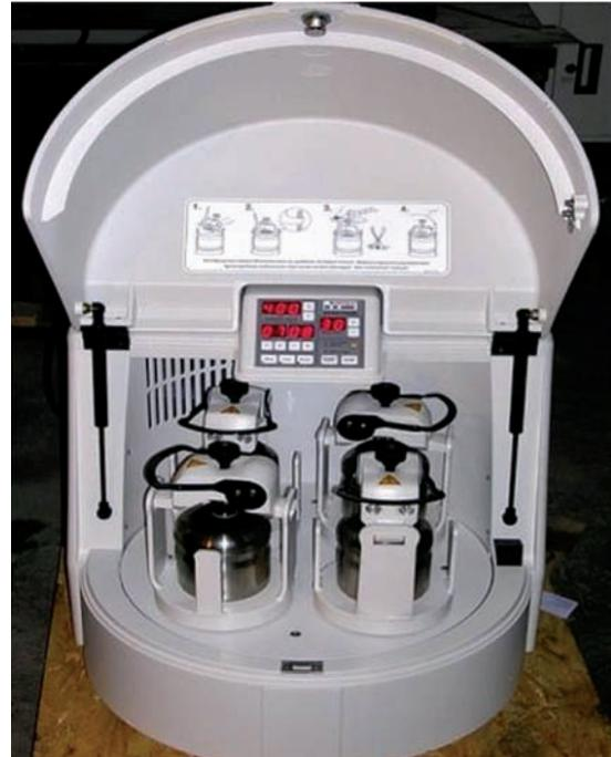
**Fig. 3: Planetary ball mill used for mixing of starting powders**
