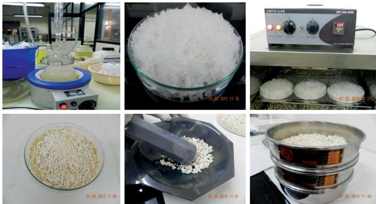
Fig. 1: Preparation scheme of PHOA
