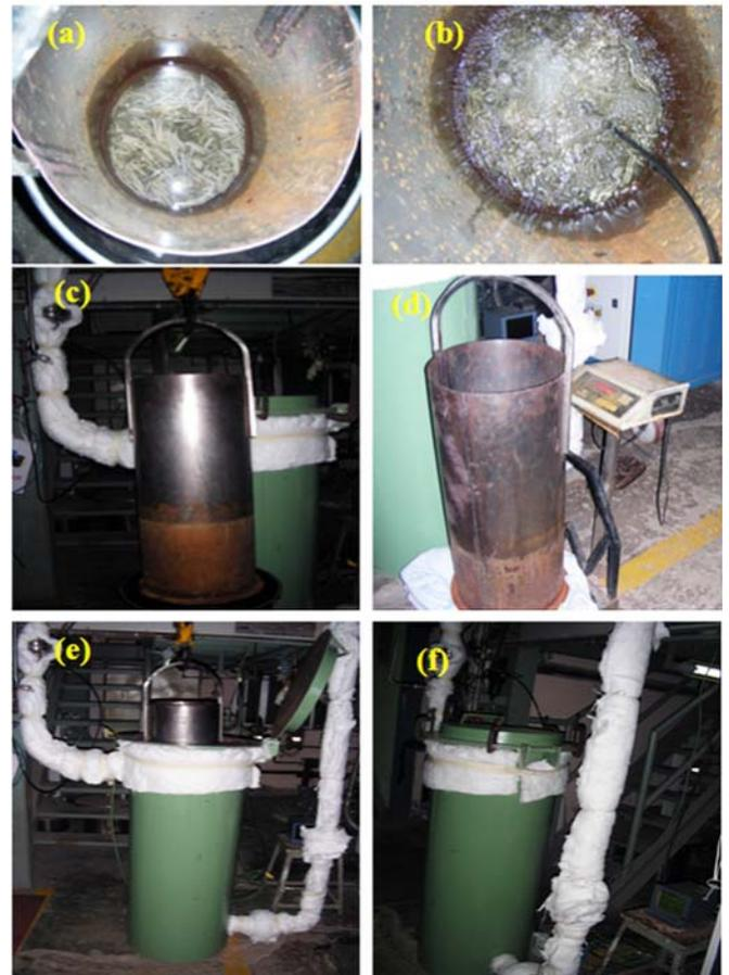
**Fig. 2: Experimental stages – (a) immersion of hull pieces in the water, (b) air sparging, (c) water dripping, (d) weighing, (e) loading of hull batching can inside dryer, and (f) closing of lid with C clamps.**
