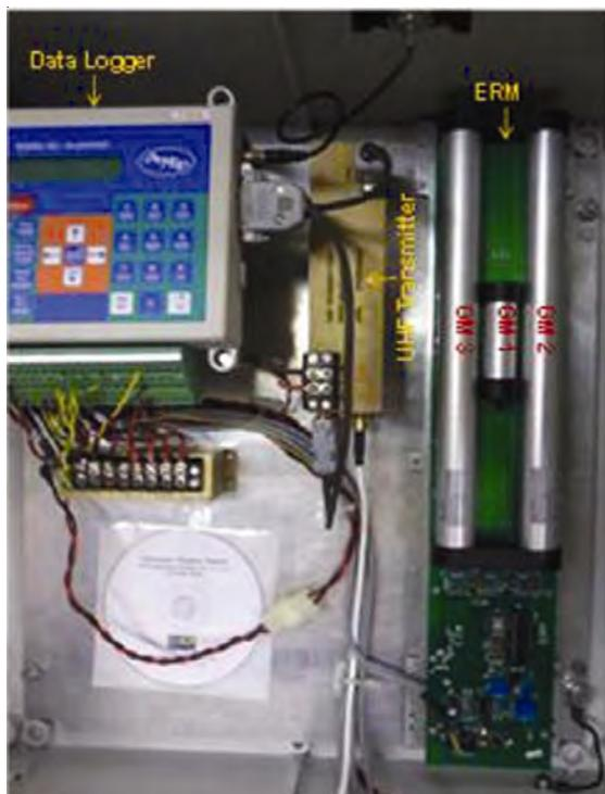
Fig. 2 ERM in waterproof multi-purpose box of ERM-AWS system along with Data Logger and UHF Transmission facility
