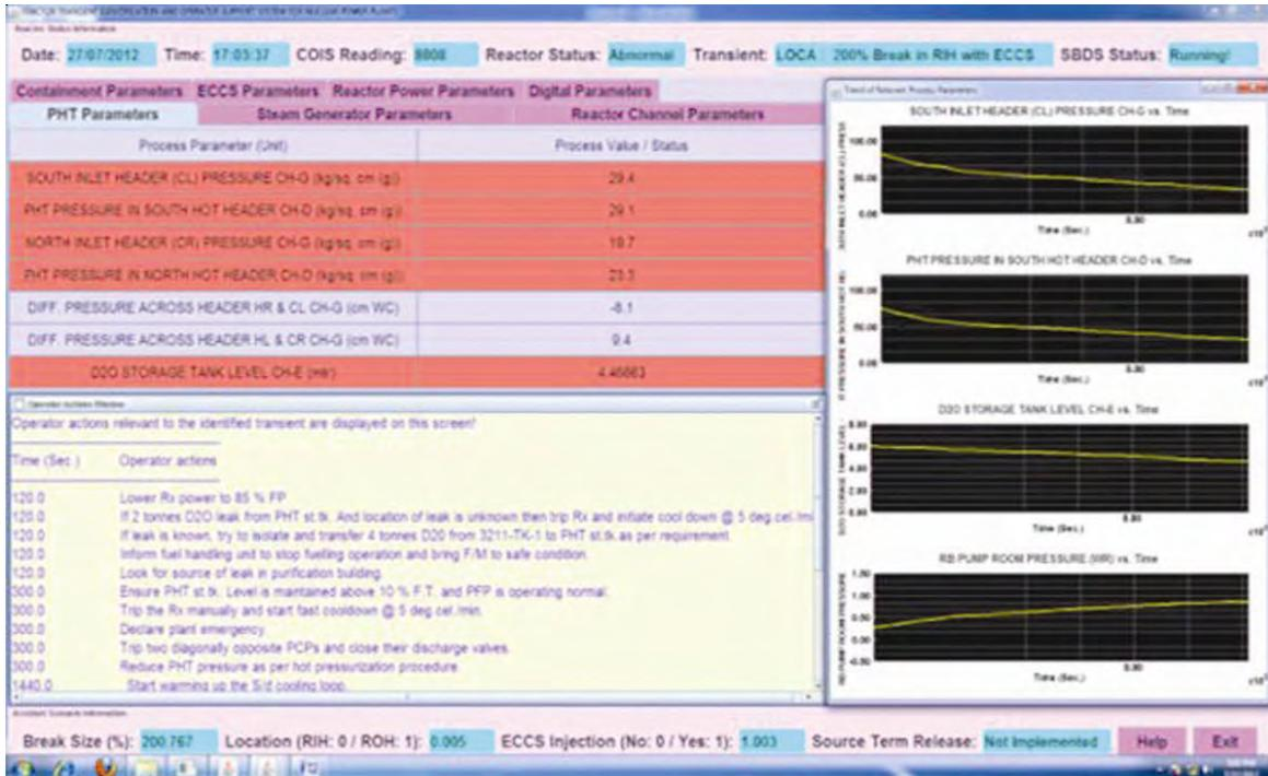
Fig. 10: Diagnostic system output for LOCA scenario
