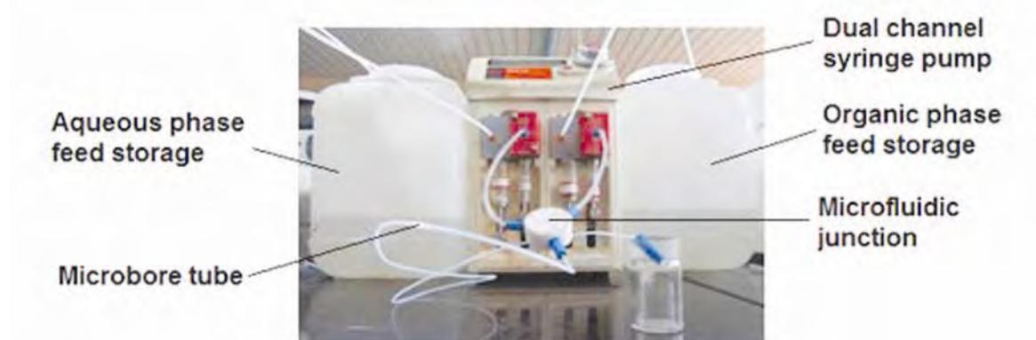
Fig. 1: Experimental setup used in the experiments with single microbore tubes
