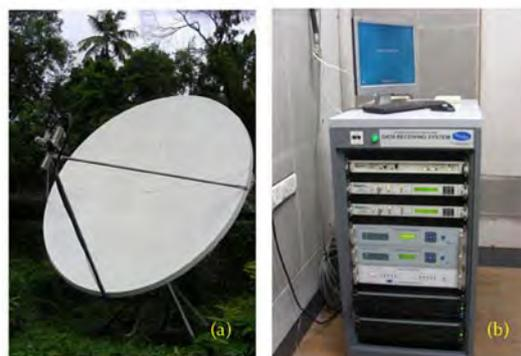
Fig. 3 Data receiving Earth Station at Anushaktinagar (a) 3.8 meter Receiver with Antenna (b) data Server
