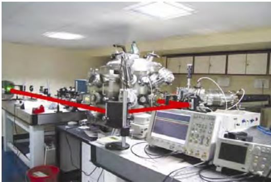
Fig. 6: Photograph of experimental chamber. Red line shows path of the main laser beam in the chamber.
