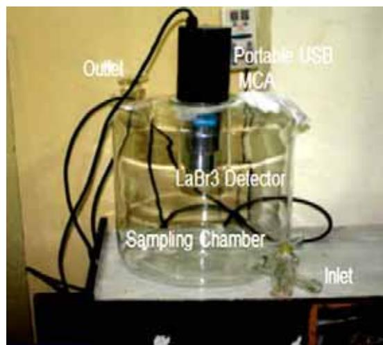
Fig. 6: Thoron sampling chamber
