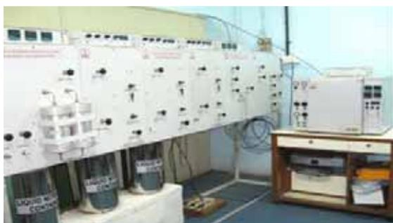
Fig. 7: Photograph of chromatography system for rare gas separation
