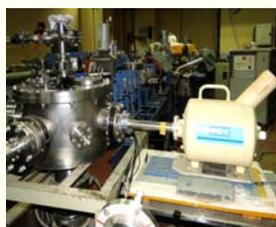
Fig. 2: PIGE set up at FOTIA: Beam chamber and HPGe detector
