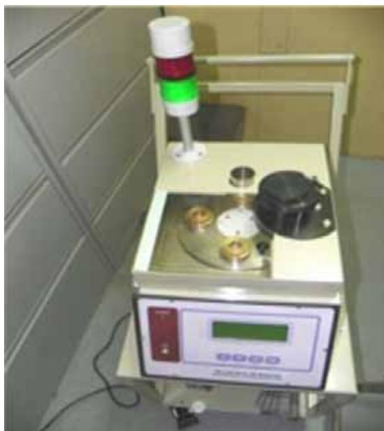
Fig.10: Online spot air sampler
