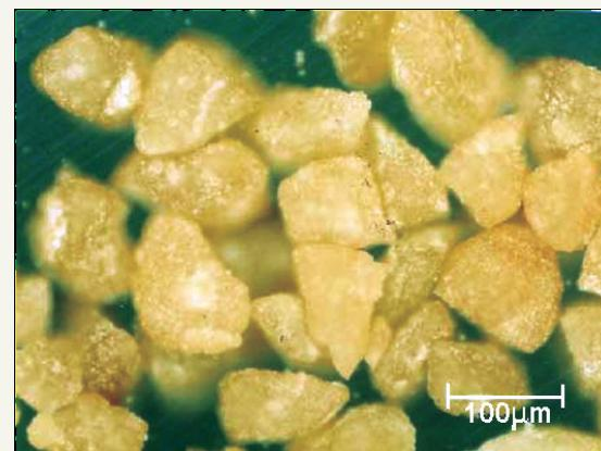
Fig. 2: Particle morphology of sintered  $\text{GdAlO}_3$  granules
