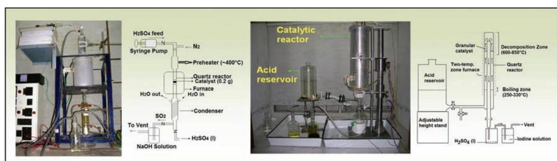
Fig. 1: Sulfuric acid decomposition setups: (A) For powder catalyst, (C) For granular catalyst. (B) and (D) are the schematics of setup (A) & (C).
