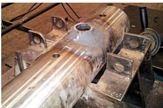
Fig. 14: Component with nozzle pulled-out
