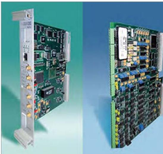
Fig. 6: Machinery protection module (MPM) and Input output module (IOM) of MPS
