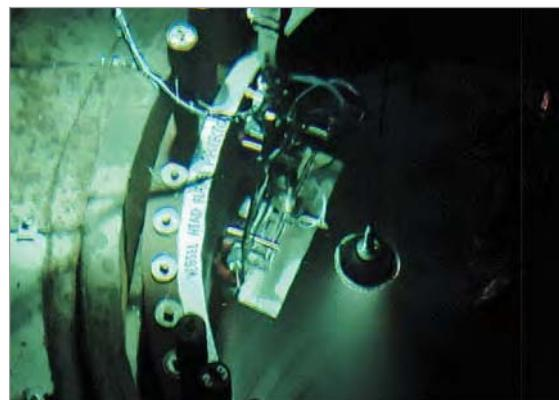
Fig. 16: WIM performing weld inspection using horizontal probe holder
