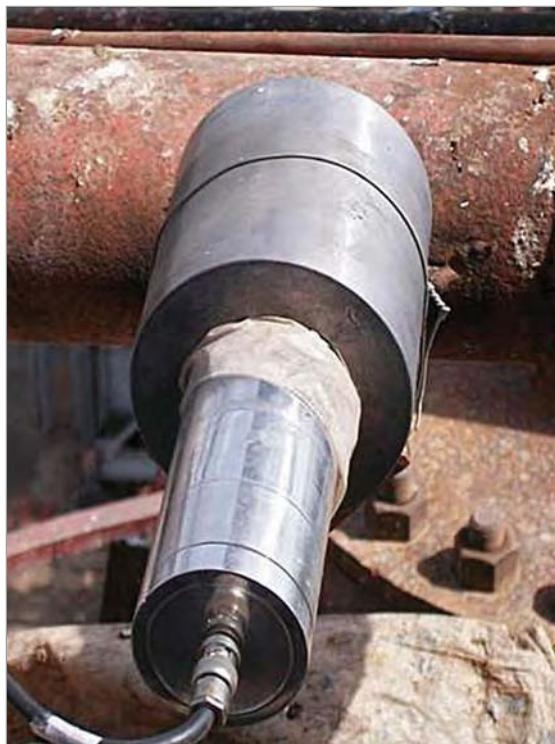
Fig. 3: Collimated scintillation detector
