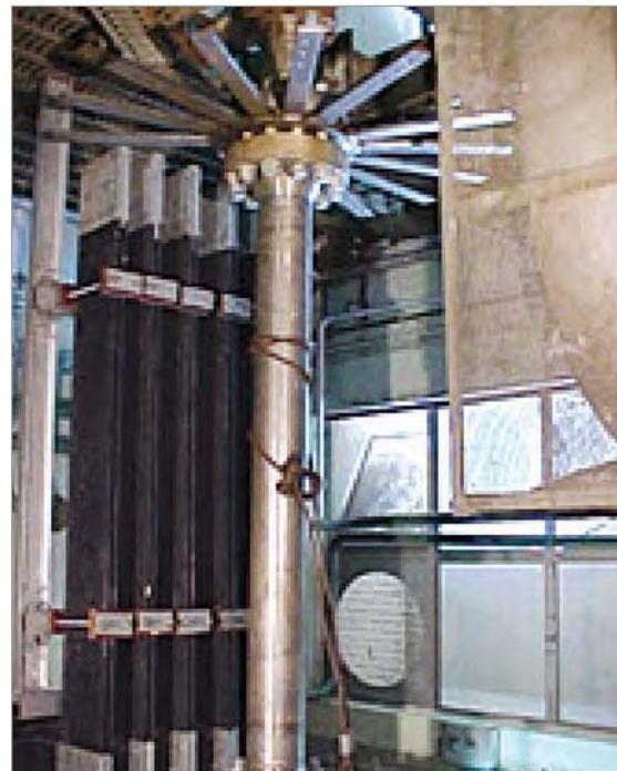
Fig. 12(a): Directly heated type FRCS with bus bar connections
