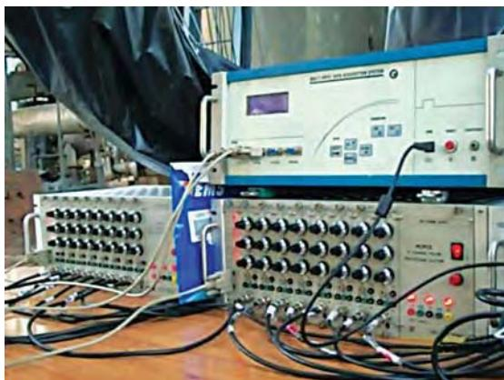
Fig. 4: Multi-input data acquisition system (MIDAS)
