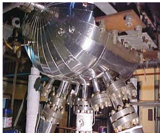
Fig. 12(b): Installed steam drum with tailpipe & downcomer connections for ITL
