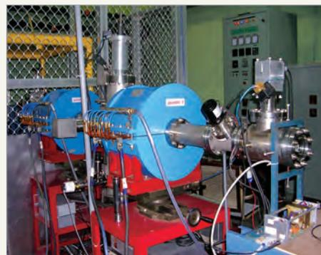
Fig. 4: LEBT test bench with solenoid magnets
