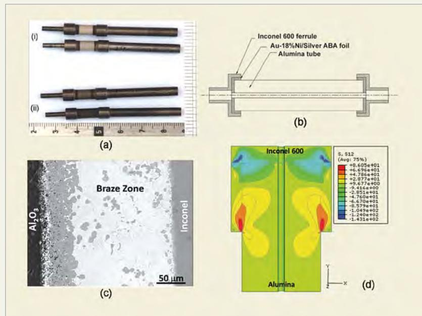
Fig. 1 (a) Alumina-Inconel 600 joints in (i) as-brazed and (ii) annealed conditions, (b) schematic diagram showing arrangement of the joint assembly, (c) microstructure of the cross-section, and (d) distribution of the residual shear stress  $t_{12}$ .
