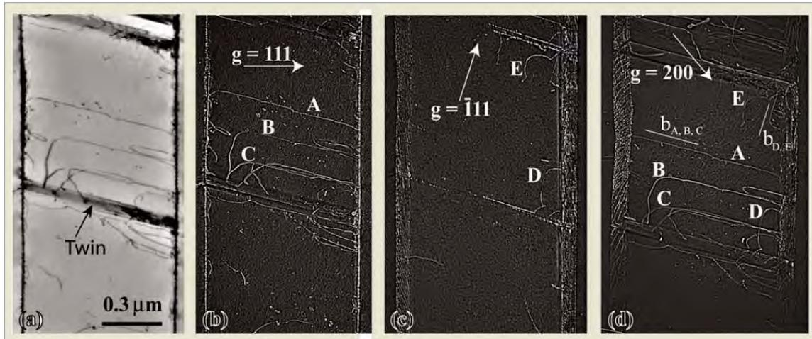
Fig. 3: (a) BF and (b) to (d) WB micrographs showing dislocations in association with twins in a  $\gamma$  lamella of  $\gamma$ -TiAl alloy deformed at 600°C. Imaging vectors are marked
