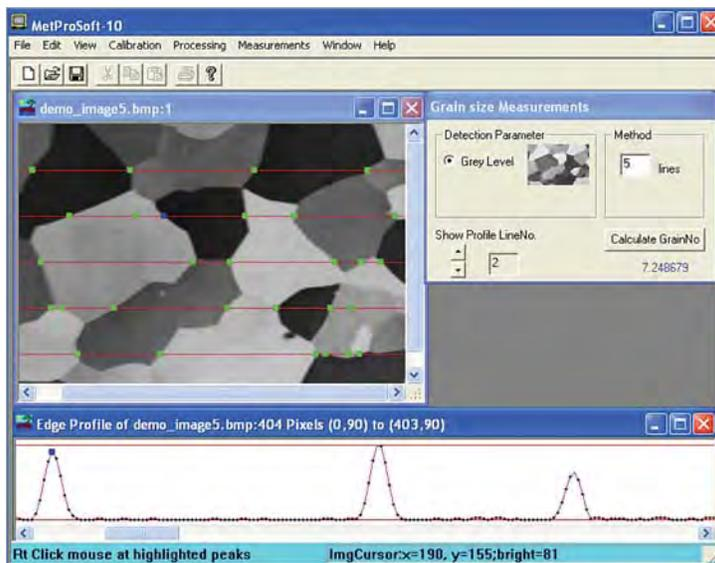
Fig. 6: Grain Number Measurement
