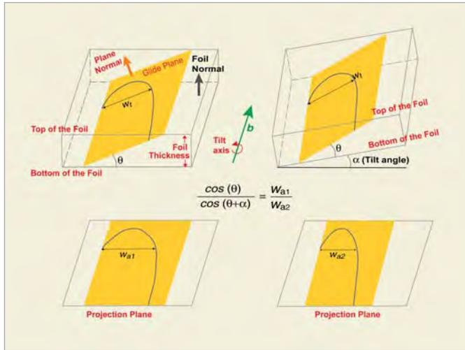
Fig. 4: Schematic illustrating the determination of habit plane of dislocation using tilt experiments.
