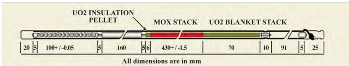
Fig. 5: Schematic drawing of FBTR MOX fuel pin
