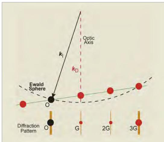
Fig. 2: Ewald sphere and positions of Kikuchi lines for the  $3g$  diffraction conditions [3].
