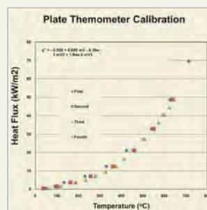
Calibration of Plate Thermometer (PT) in Cone Calorimeter
