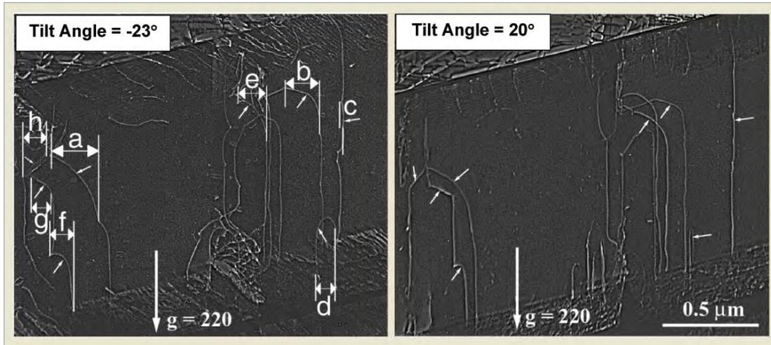
Fig. 5: WB analysis of planes containing dislocations. The habit planes of segments a to h are identified (see text for details)
