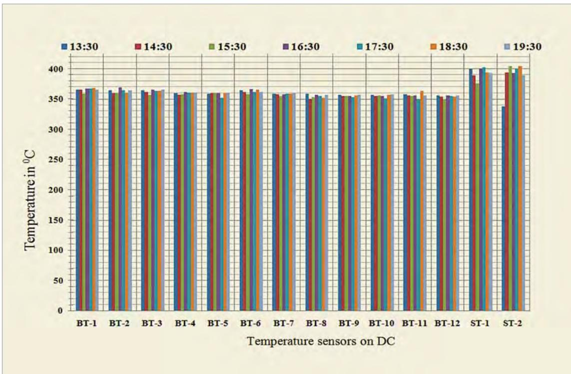
Fig. 4: Temperature Profile inside Denitration Column with 42 lph of ammonium nitrate feed. B is bed temperature at different axial locations, S is wall surface temperature
