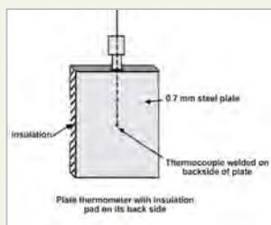
Plate Thermometer with Insulation Back Pad
