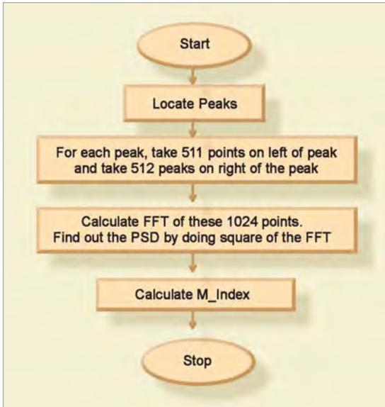
Fig. 6: Flow chart for calculation of MI
