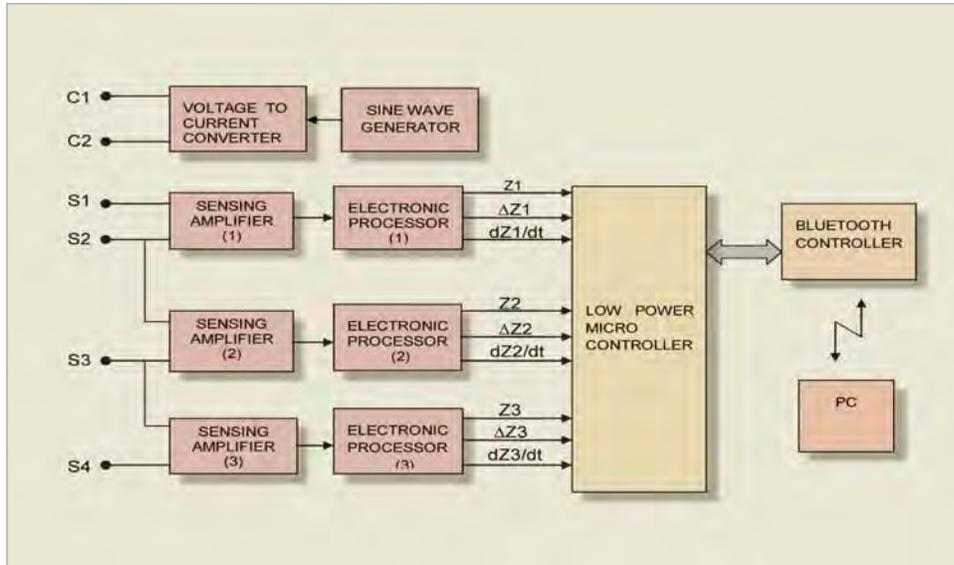
Fig. 8: shows the schematic diagram of the Peripheral Pulse Analyzer developed at Electronics Division BARC
