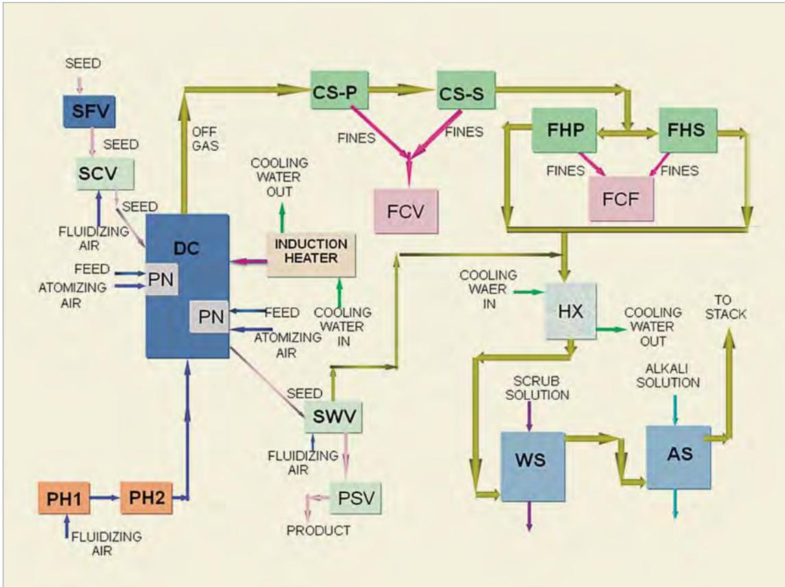
Fig. 1: Typical Block Diagram for Denitration plant
