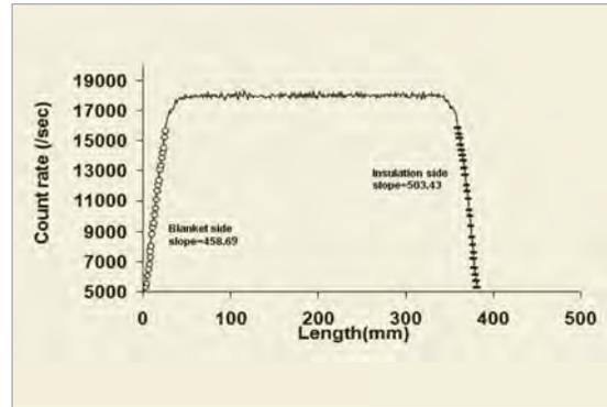
Fig.4: Gamma scan of a PHWR MOX pin with variation in PuO<sub>2</sub> content in the stack
