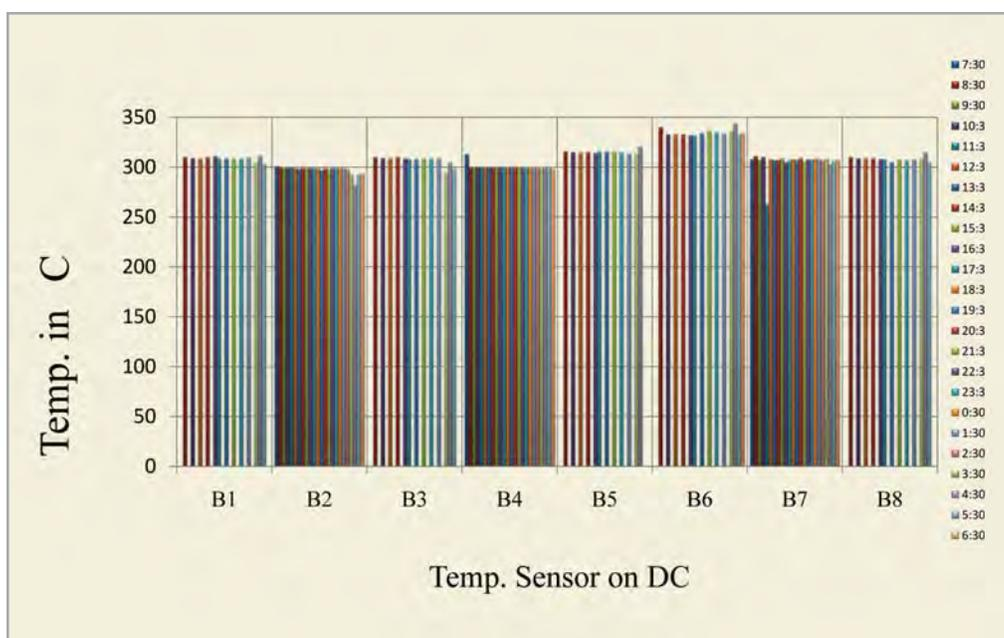
Fig. 2: A typical temperature profile inside the denitration column. B is bed temperature at different axial locations.
