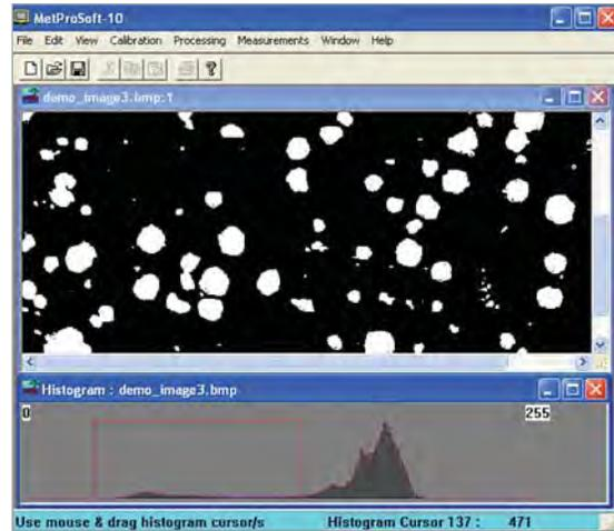
Fig. 3: Interactive Thresholding
