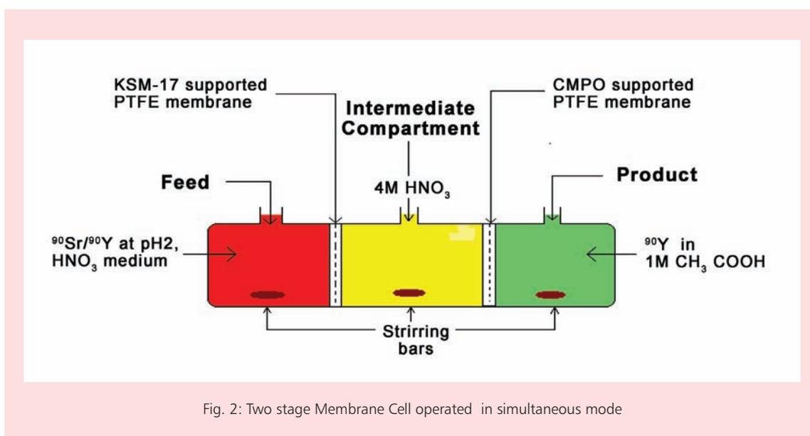
Fig. 2: Two stage Membrane Cell operated in simultaneous mode
