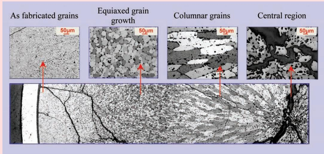
Fig. 18 Restructuring in fuel occurs due to a steep temperature gradient from the centre to the periphery of the fuel. Boundaries of the microstructural regions in an irradiated  $UO_2$  fuel can be used as markers for estimation of fuel centre temperature attained during operation.
