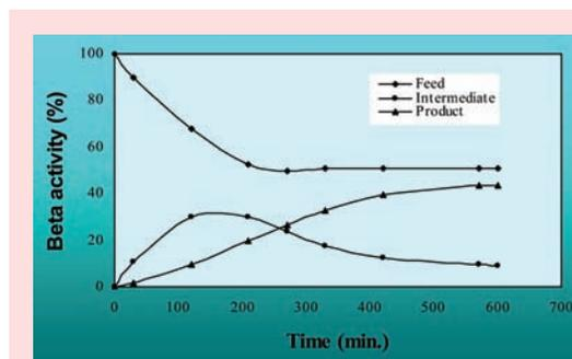
Fig. 3: Separation of  $^{90}\text{Y}$  from  $^{90}\text{Sr}/^{90}\text{Y}$  mixture using a two stage SLM system
