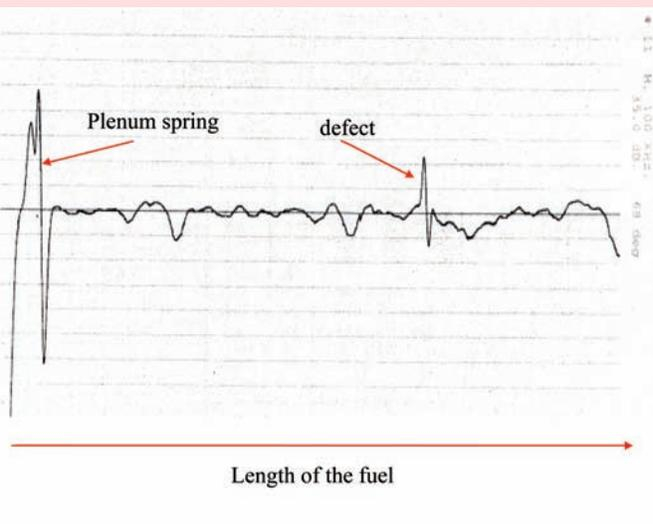
Fig. 7b: Signal obtained from a defect in the fuel cladding.
