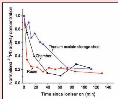
Fig. 1: Variation in the activity concentration of <sup>212</sup>Pb in the room, chamber and field environments
