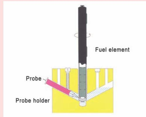
Fig. 5b: Fuel pin in the probe holder unit.
