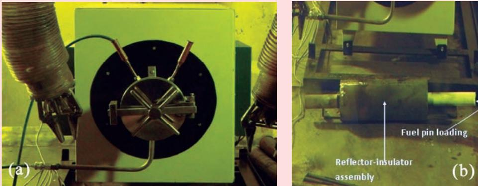
Fig. 13: Furnace used for ballooning studies on irradiated fuel
