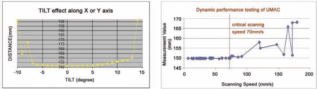
Fig 2: Experimental qualification of UMAC sensor under operating condition of FM tilt and FM scanning speed
