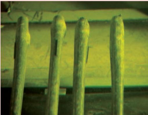
Fig. 13c: Some of the ballooned fuel elements are shown.
