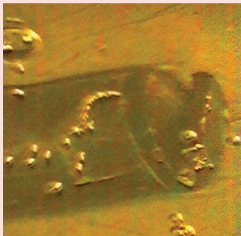
Fig. 4a: Nitrogen gas bubbles coming out of the leak in the end cap weld.
