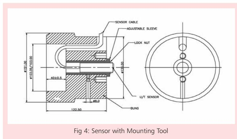
Fig 4: Sensor with Mounting Tool
