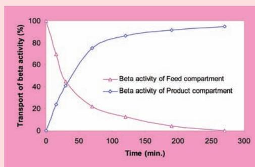
Fig. 5b: Transport of  $^{90}\text{Y}$  in 2<sup>nd</sup> Stage at 100 mCi Level
