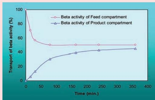
Fig. 5a: Transport of  $^{90}\text{Y}$  in 1<sup>st</sup> Stage at 100 mCi Level
