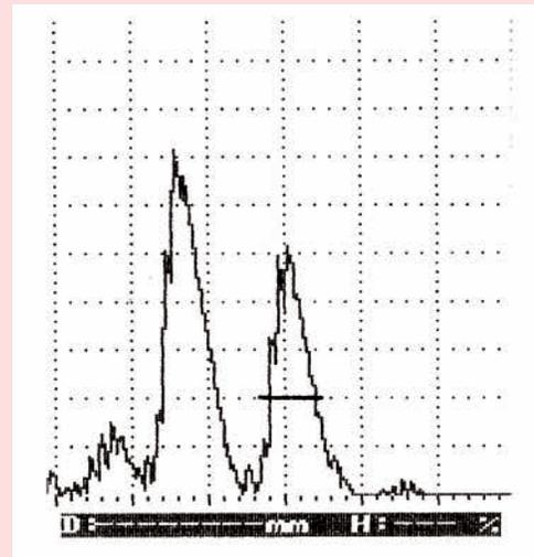
Fig. 5d: Signal from a defective weld with partial fusion
