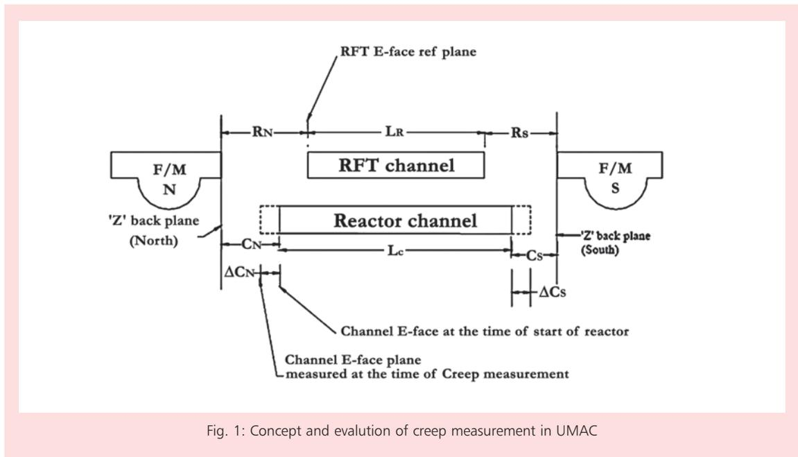
Fig. 1: Concept and evaluation of creep measurement in UMAC
