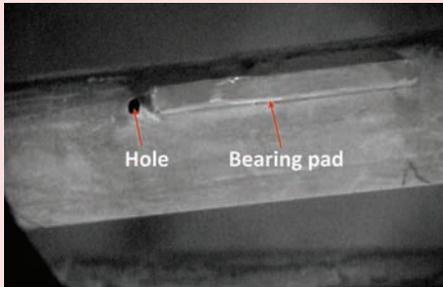
Fig. 3d: Pinhole due to damaged bearing pad from bundle no. 102653
