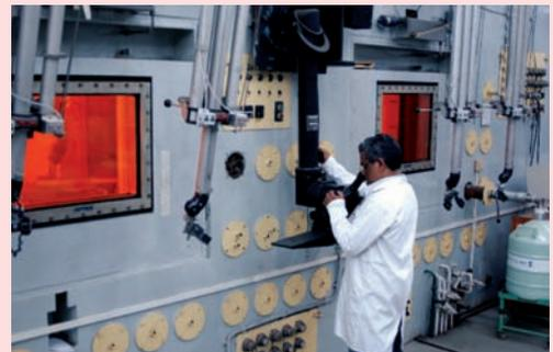
Fig. 3a: Wall periscope for visual examination in hot cells facility.
