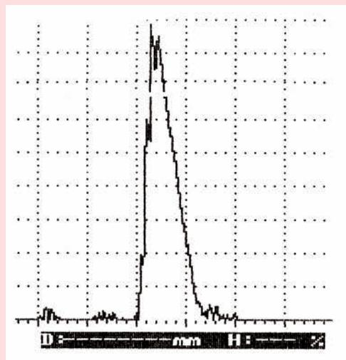
Fig. 5c: Weld step signal from a sound end cap weld
