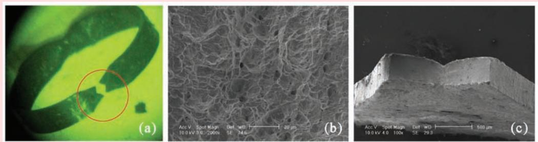
Fig. 12: Deformation behaviour of clad after burnup level of above 15000 MWd/tU at 583 K showing (a) significant level of ductility (b) failure by void formation in the central portion of specimen followed by (c) localized shearing at 45° to the loading direction.
