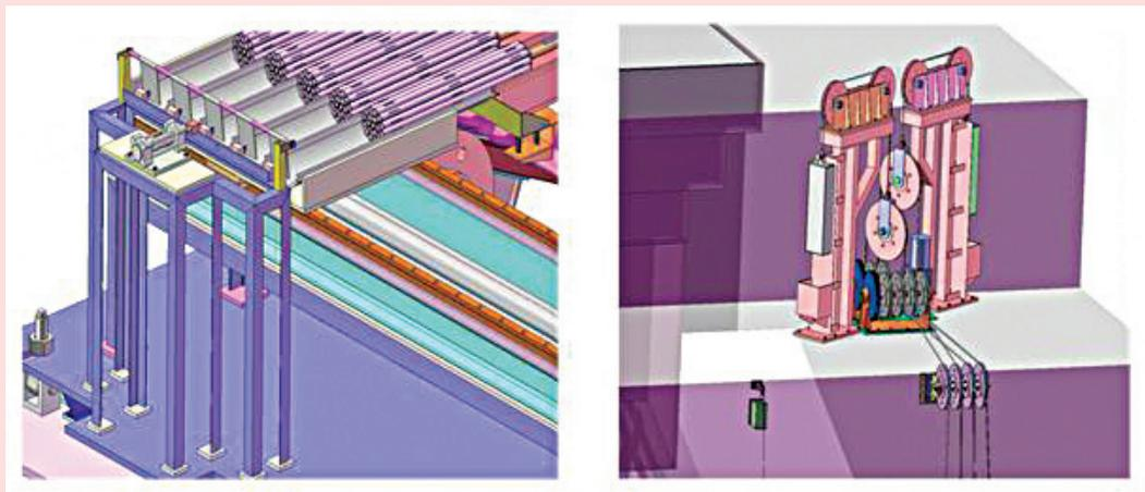
(f) Direct Sensing of Fuel Bundles on X-Table (g) Counter Weight Arrangement
