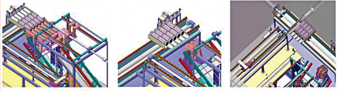
(a): Pusher-I Sub-assembly (b) X-Table Sub-assembly (c) Pusher-II Sub-assembly
