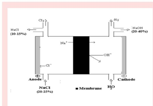
Fig.5: Schematic representation of chlor alkali electrolyzer.
