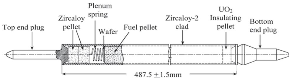
Fig. 14: A typical experimental fuel pin for MOX irradiation
