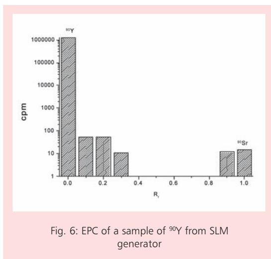
Fig. 6: EPC of a sample of  $^{90}\text{Y}$  from SLM generator
