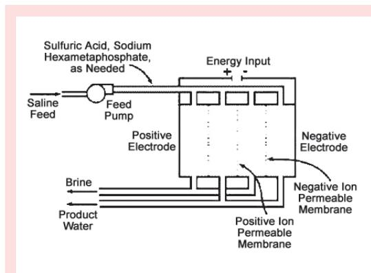
Fig.4: Electrodialysis setup
