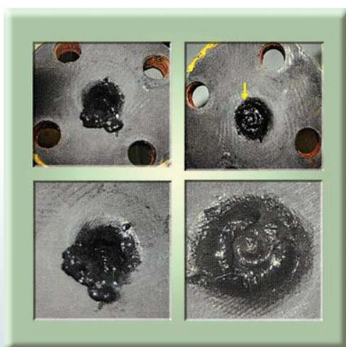
**Fig. 1: Clogged pipeline with fungal biomass**
