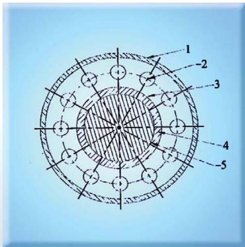
**Fig. 2a: Cross section of the pumping geometry of 38mm Nd:Glass amplifier.**
