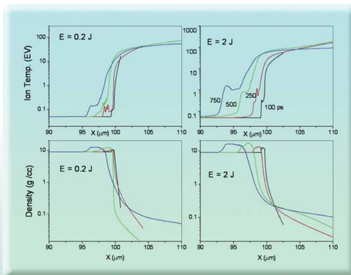
**Fig. 8: Spatial profiles of ion temperature and density for laser energy 0.2 Joule and 2 Joules**
