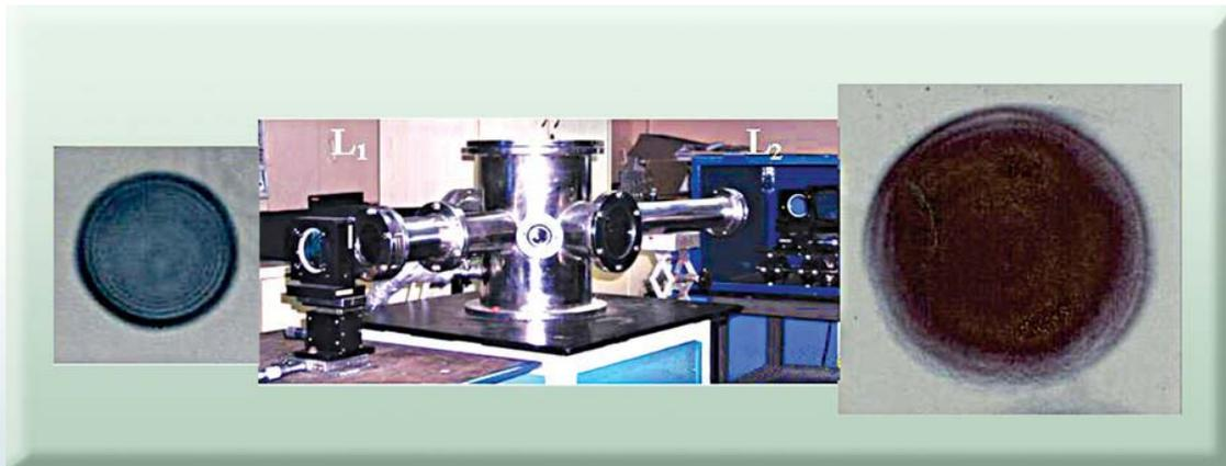
Fig. 3: Spatial filter assembly with beam before the spatial filter and after the spatial filter
