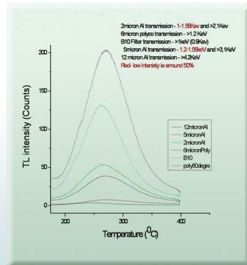
**Fig. 12: Glow curve of TLD ( $\text{CaSO}_4:\text{Dy}$ ) with various filters**
