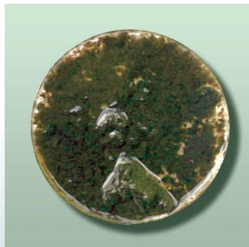
**Fig. 2: Biomass collected from fouled pipeline**
