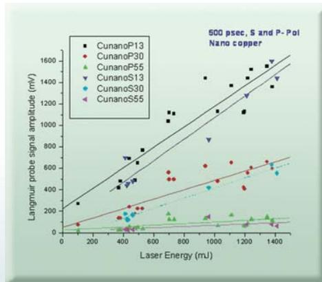
**Fig. 11: (contd.)** Scaling of ion densities and ion velocities with laser pulse energy for two polarization measured by set three of Langmuir probes placed at various angles.
