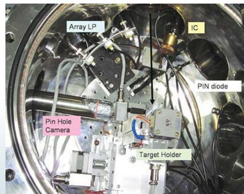
Fig. 7b: Vacuum chamber: inside view
