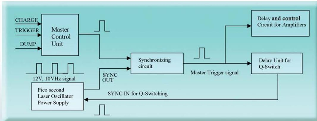
Fig. 6: Schematic of Laser Electronics System
