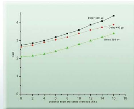
**Fig. 2b: Radial gain variation of 38 mm Nd:Glass**
