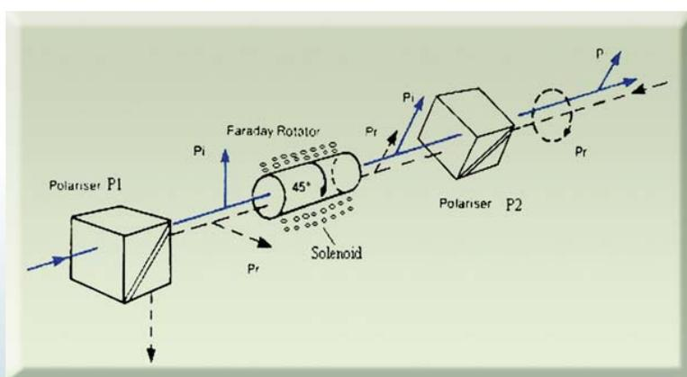
Fig. 4a: Schematic of Faraday isolator
