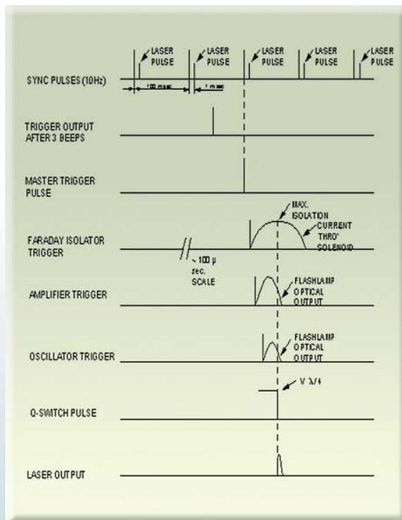
Fig. 5: Timing sequence for various trigger pulses
