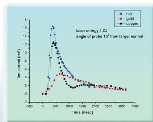
Fig. 10: Ion current recorded by Langmuir probe
