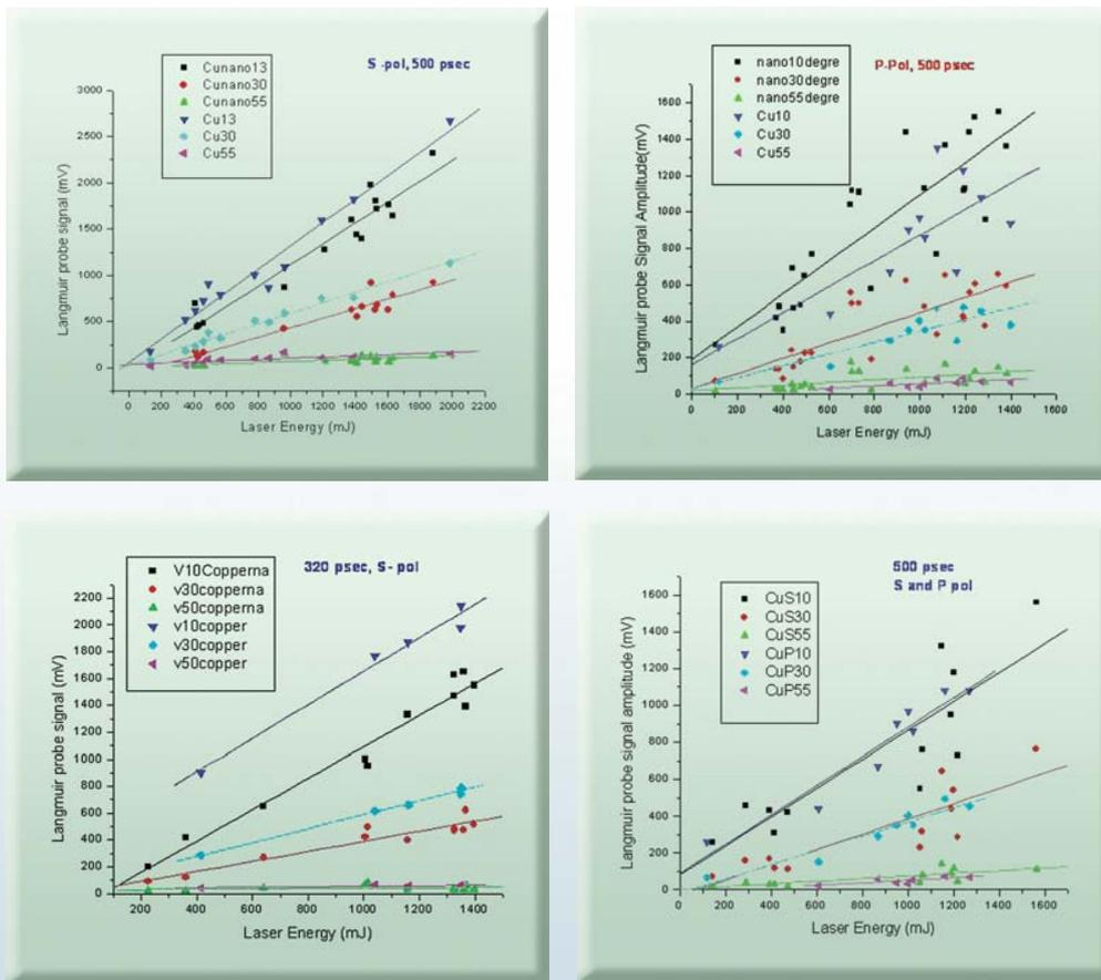
**Fig. 11: Scaling of ion densities and ion velocities with laser pulse energy for two polarization measured by set three of Langmuir probes placed at various angles.**
