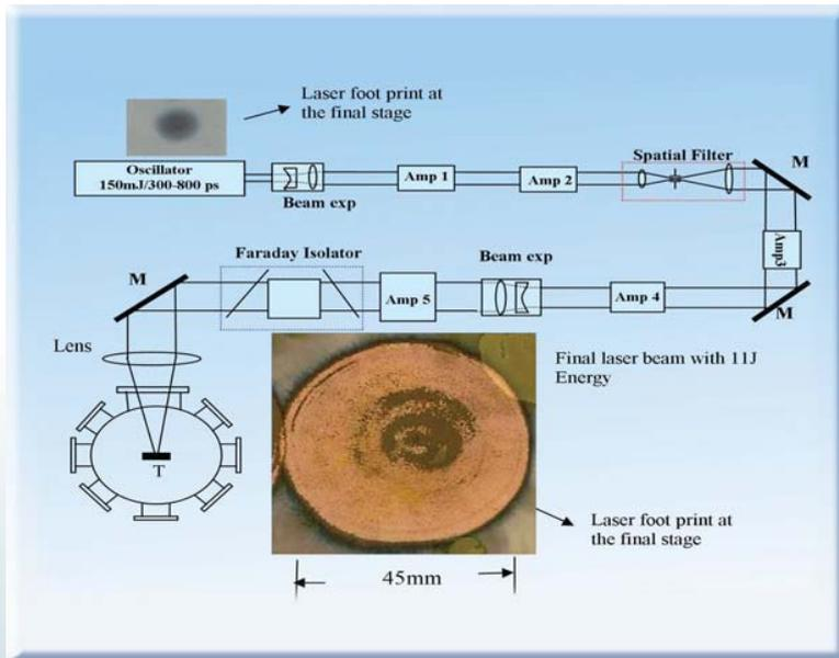
Fig.1a: 10J/300-800 psec laser chain: schematic
