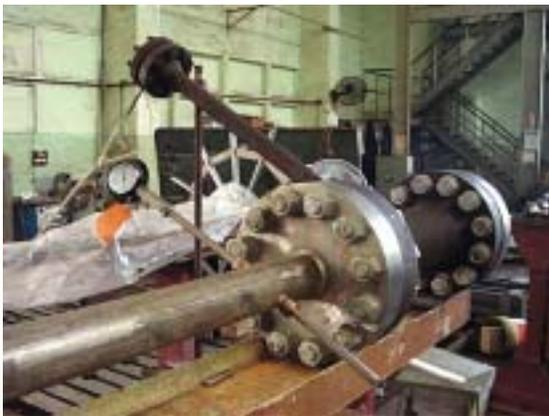
Fig.4: FRCS channel assembly under hydro-testing
