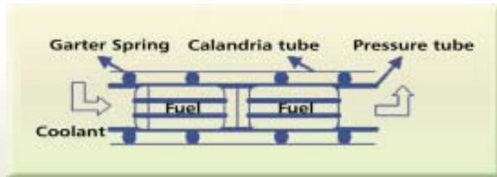
Fig. 1: Simplified sketch of coolant channel
