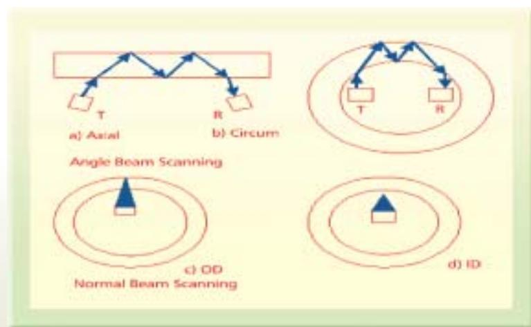
Fig. 3 : Angle and normal beam scans
