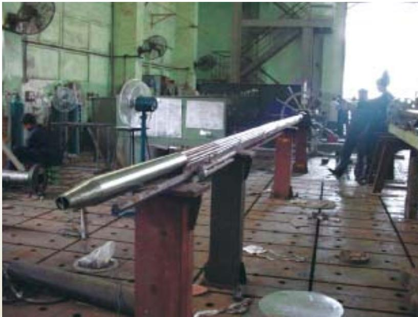
Fig 2: SS tube plate end of fuel rod cluster
