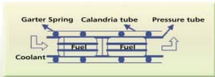
Fig. 1: Simplified sketch of coolant channel
