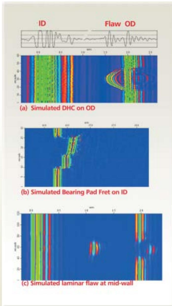
Fig. 5: B-scan images of simulated flaws in pressure tube samples
