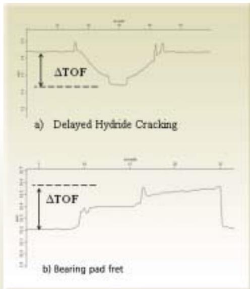
Fig. 6: Time-of-flight plots for simulated flaws in pressure tube
