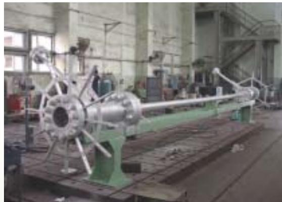
Fig:5 : Full FRCS assembly ready for despatch
