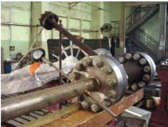
Fig.4: FRCS channel assembly under hydro-testing
