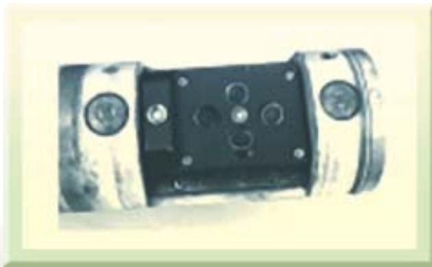
Fig. 2: Inspection head for pressure tube examination
