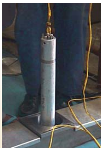
Fig. 8: Dummy element with accelerometer is being dropped into the guide tube
