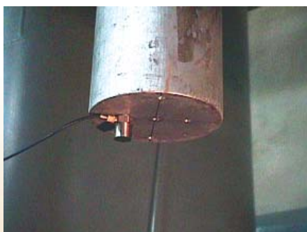
Fig. 9: Accelerometer attached to the bottom side of the guide tube
