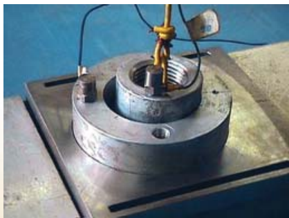
Fig. 7: Accelerometer attached to the dummy element and the top side of the guide tube
