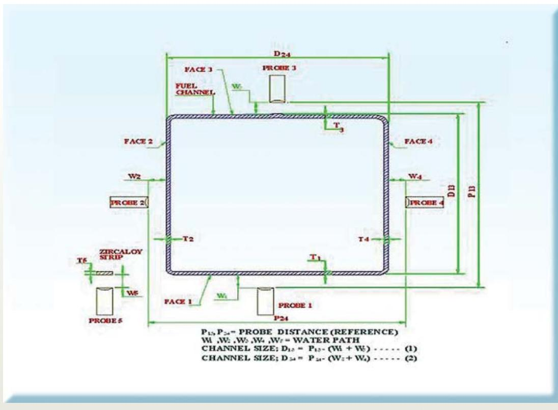
proper velocity the input wall thickness of channel can be measured, by selecting either first interface and first back wall echo or first and second back wall echoes, from the channel. However, switching from water path measurement to wall thickness measurement, requires change of range, gain, damping and other parameters, suitable for measuring 1.5 mm thick zircaloy.
