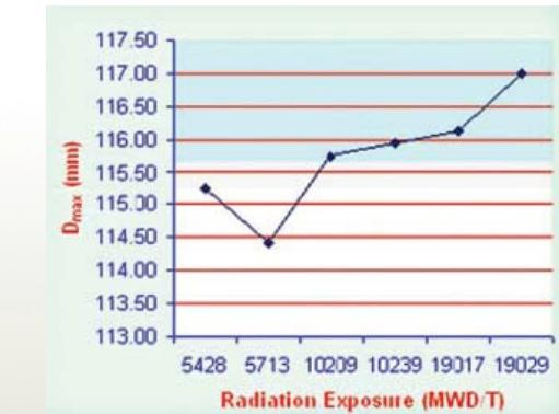
Fig. 7: Channel growth versus exposure
