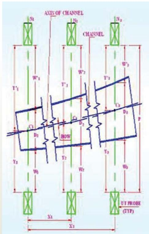
Fig. 2: Bow measurement by CGMD
