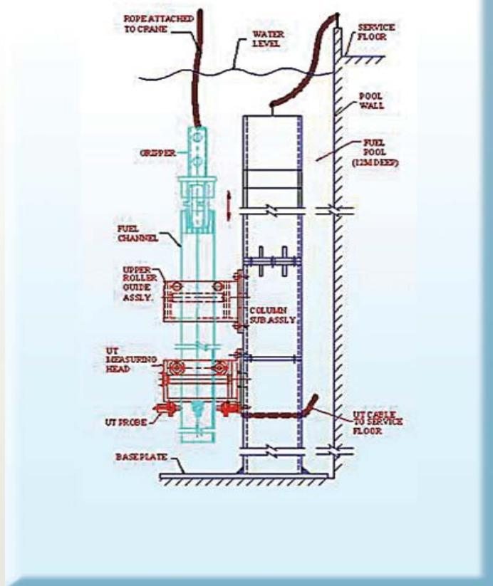
Fig. 5: Measurement set up for CGMD
