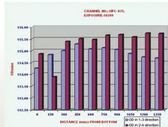
Fig. 6: OD of TAPS fuel channel by UT
