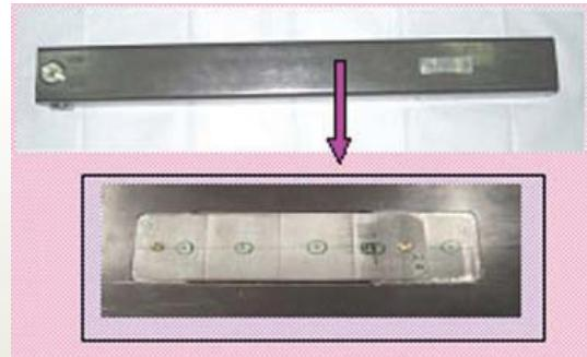
Fig. 4: Calibration sample and exploded view of step block
