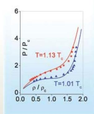
Fig. 8: Two Isotherms of Hg
