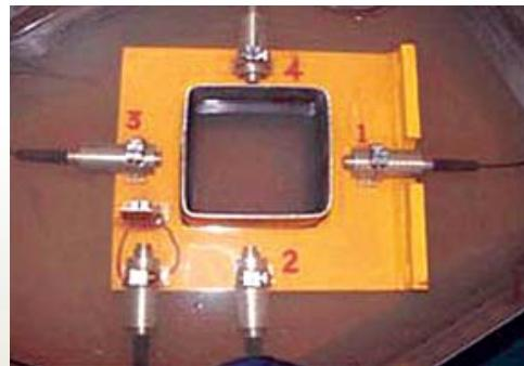
Fig. 3: Calibration check using a small tank with measuring head
