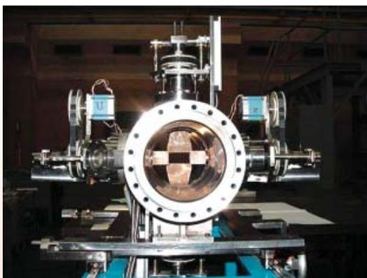
Fig. 1: Four slit jaws showing maximum opening size of 60x30mm
