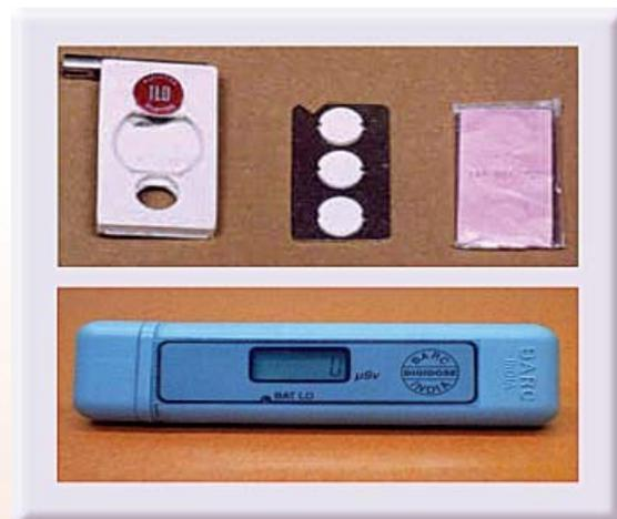
Fig. 6: Thermoluminescent Dosimeters (TLDs) and The Digital Pocket Radiation Dosimeter used for dose measurement (external exposure)
