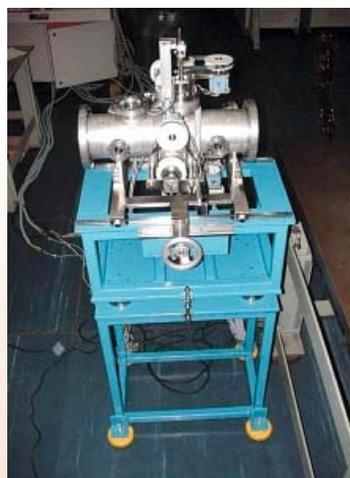
Fig. 3: Primary slit assembly
