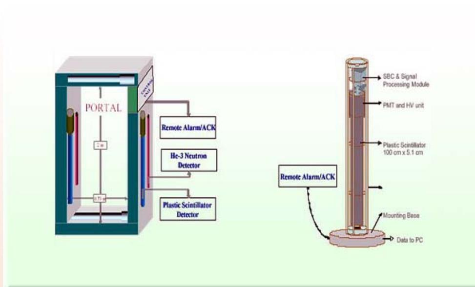
Fig. 10: Portal Monitor and Limb/Pole Monitors developed in BARC for the detection of illegal movement of radioactive materials (Gamma/Neutron)
