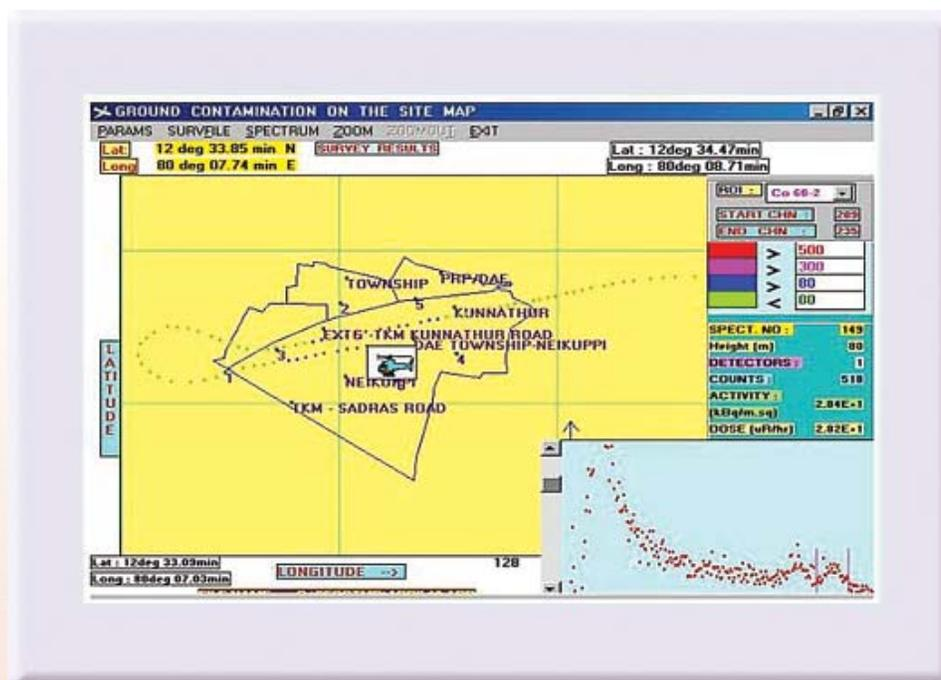
Fig. 12: Display on the PC screen during an aerial survey above simulated contamination using AGSS mounted in a MI - 8 Helicopter
