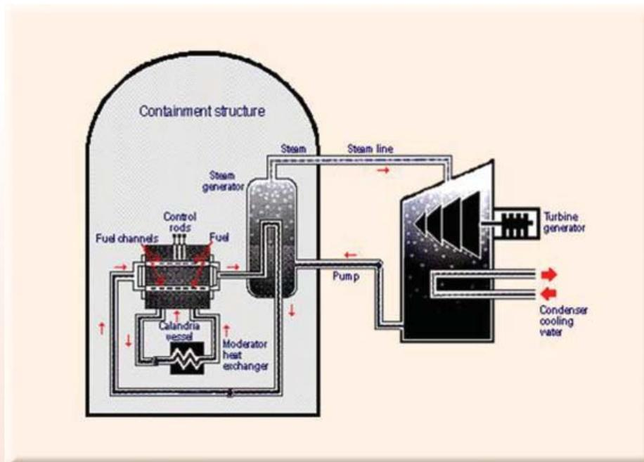
**Fig. 1: Simplified diagram of a nuclear power reactor and its containment**
