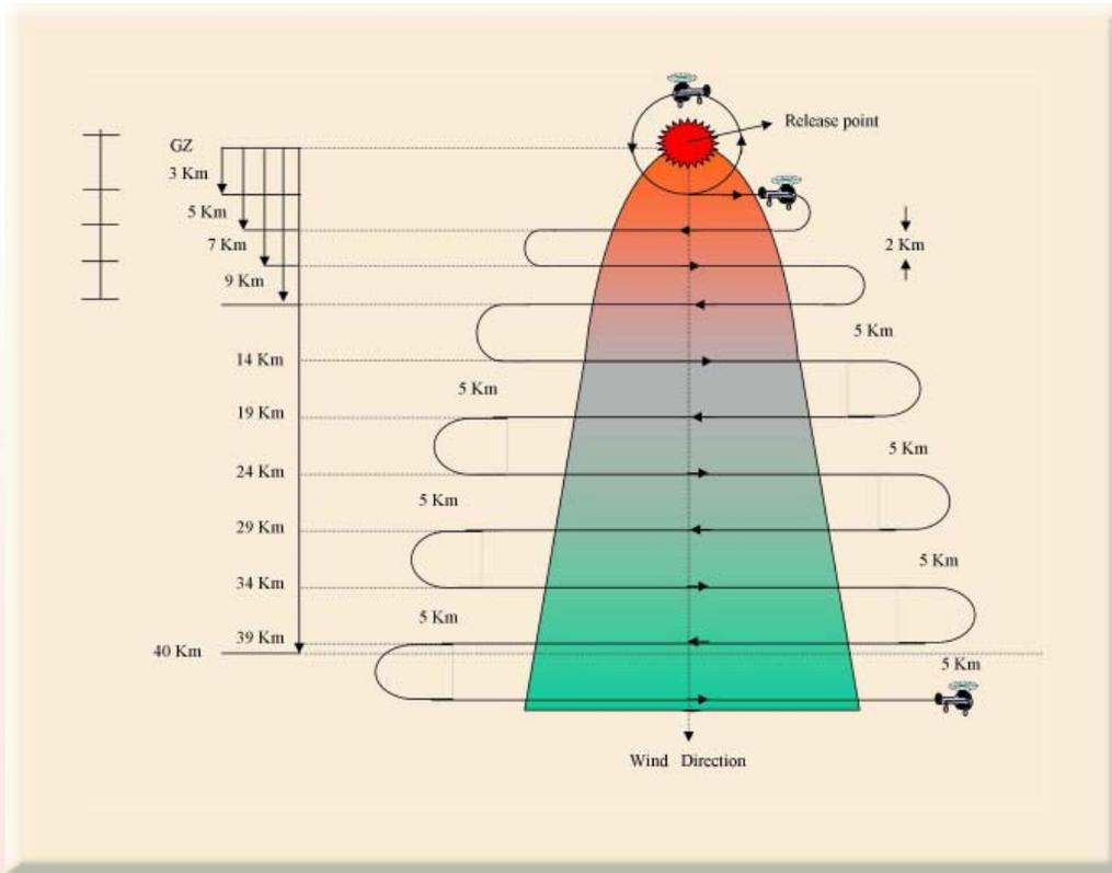
Fig.11: Aerial survey methodology for quick assessment of radiological impact (using AGSS or CARMS) in case of any accidental release of radioactivity to the environment
