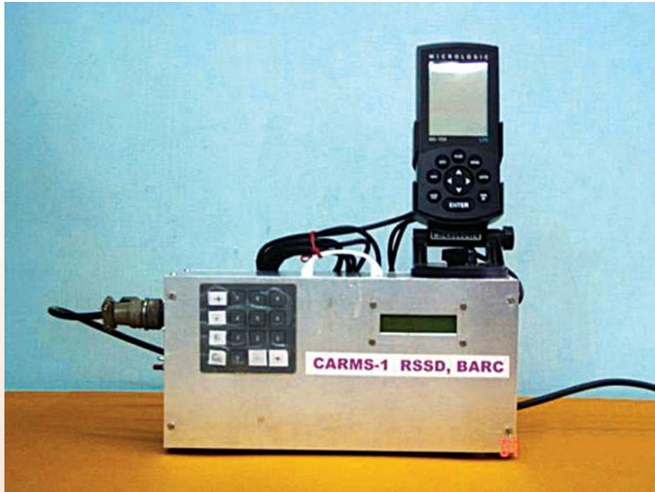
Fig. 9: Compact Aerial Radiation Monitoring System (CARMS) for quick assessment of radiological impact using UAVs
