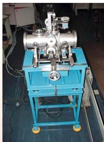
Fig. 3: Primary slit assembly
