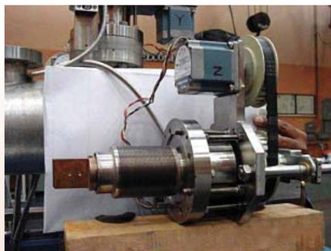
Fig. 2: Slit jaw assembly
