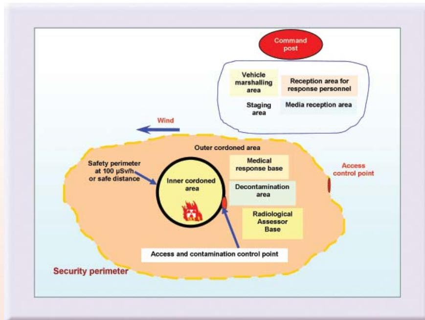
Fig. 5: Typical layout - Safety and security perimeter in case of emergencies leading to radioactive contamination
