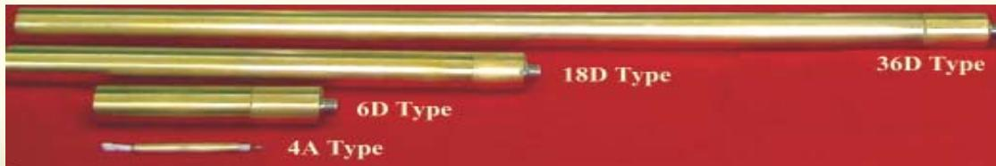
Fig.1: Some of the neutron proportional counters mentioned in Table 1
