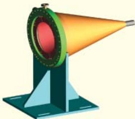
Fig. 13: Conical target for beam dump
