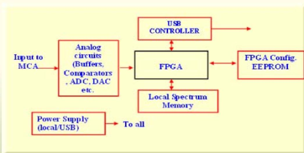
Fig. 1 : Block diagram of the MCA
