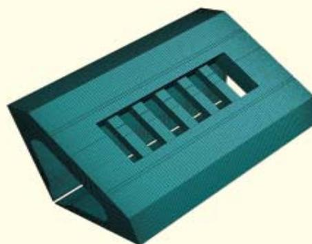
Fig. 9: RFQ cavity with vacuum port
