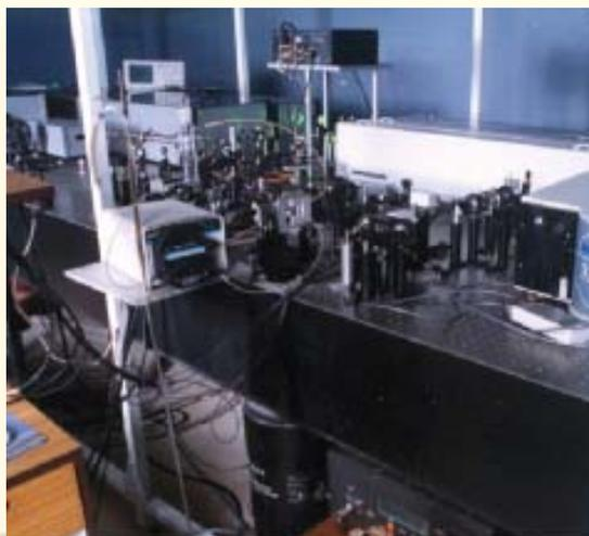
Femtosecond Transient Absorption Spectrometer
