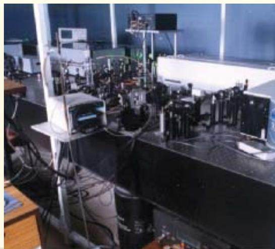
Femtosecond Transient Absorption Spectrometer
