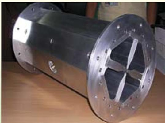
**Fig. 17b: Aluminium model of RFQ**
