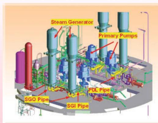
Fig. 8: Schematic of PHT System: TAPS 3 & 4
