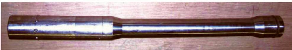
Fig. 3: Channel Flow Blocking Plug
