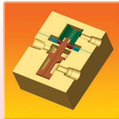
Fig. 4: Schematic cross sectional view of Constant Level Valve
