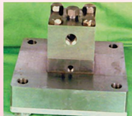
Fig. 1: Auto-Differential Pressure Control Valve
