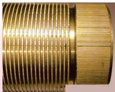
Fig. 1(b): Wear marks on B-RAM labyrinth
