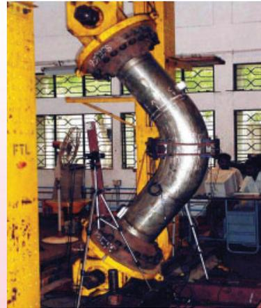
Fig. 11a: Elbow Fatigue Test Set-up
