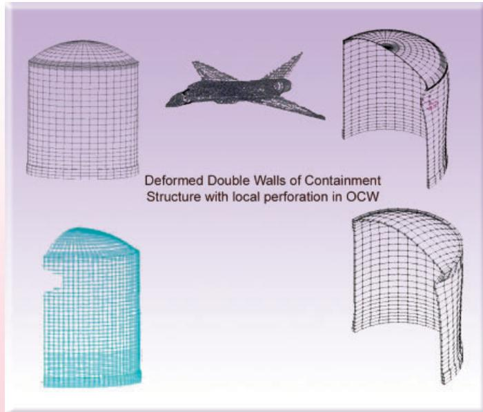
Fig. 3: Scenario during the Postulated Accidental Aircraft impact on containment structure of Tarapur 3 & 4 Plant Containment Structures
