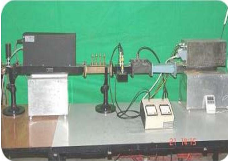
Fig. 11: Microwave Generator and the Plumbing Line
