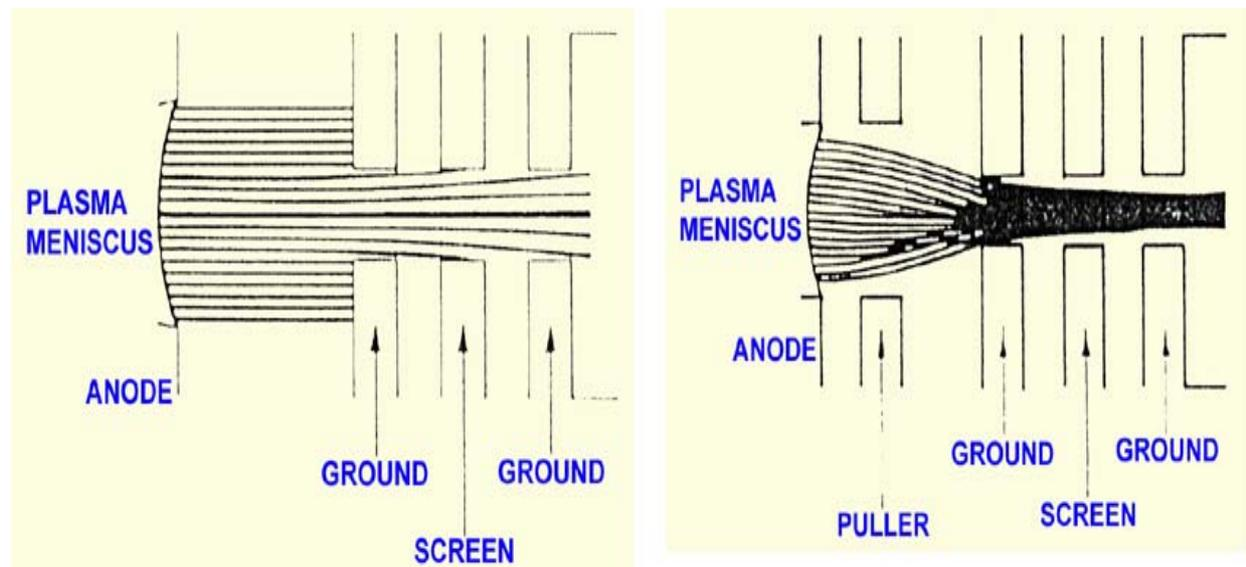
Fig. 6 Transmission of the beam through the Pentode Extraction Geometry
