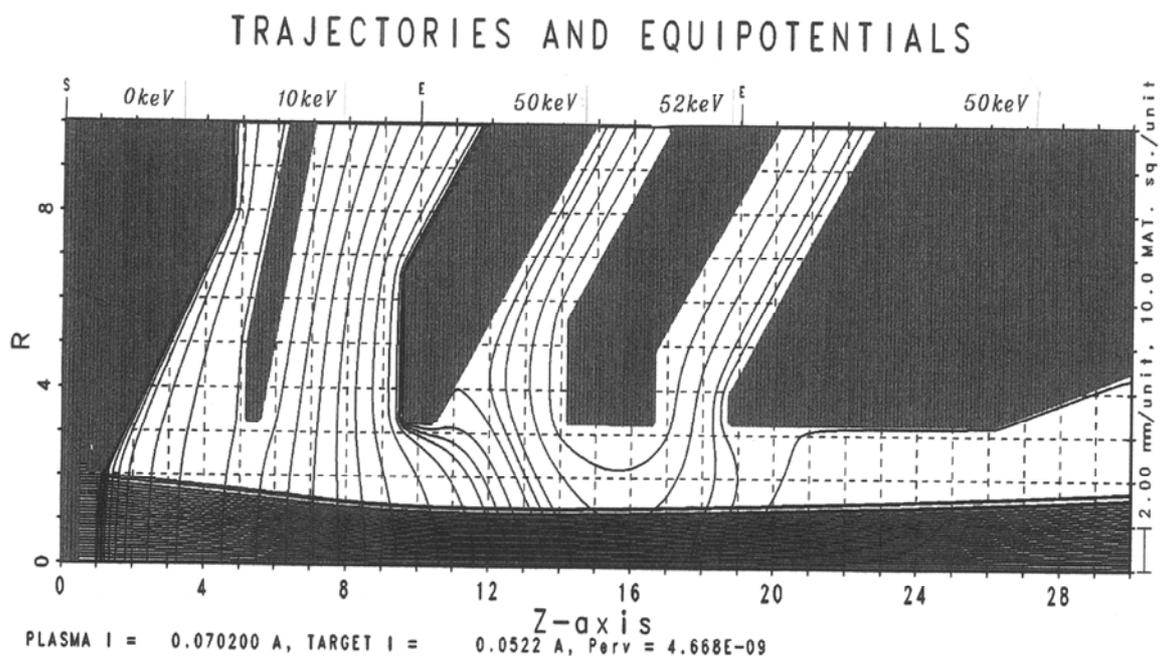
Fig. 7 Simulation of 50 keV, 50 mA beam through the Extractor Geometry
