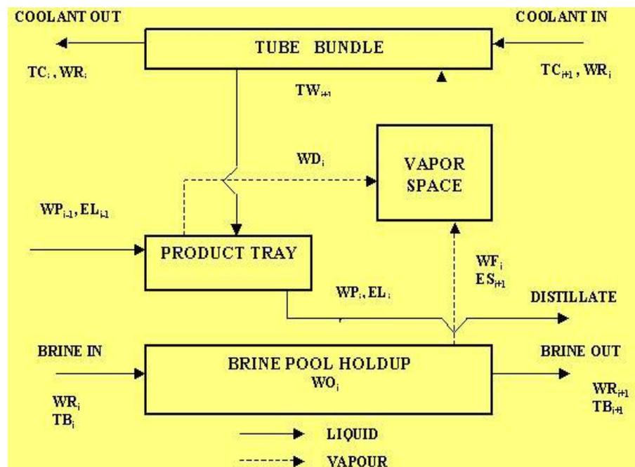
Fig. 1 Schematic of the evaporator
