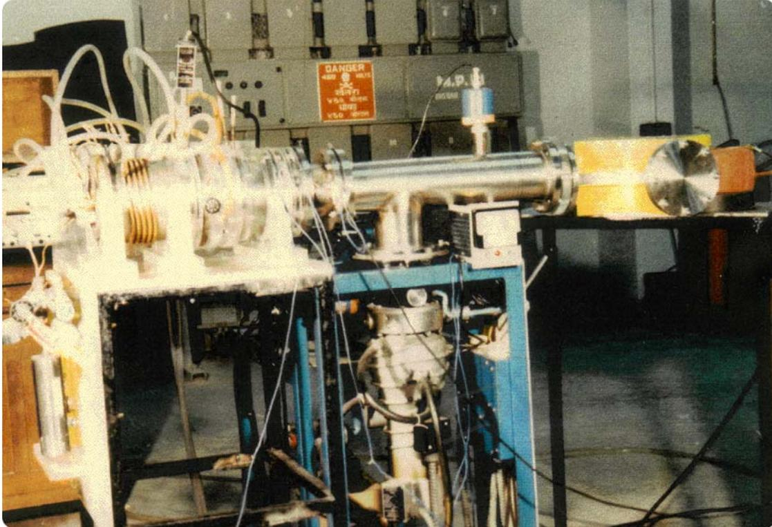
*Fig. 1 A close up view of the Duoplasmatron Ion Source*
