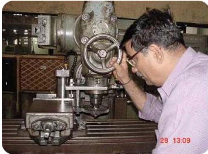
Fig.3 Inner face Counter Boring Attachment in use
