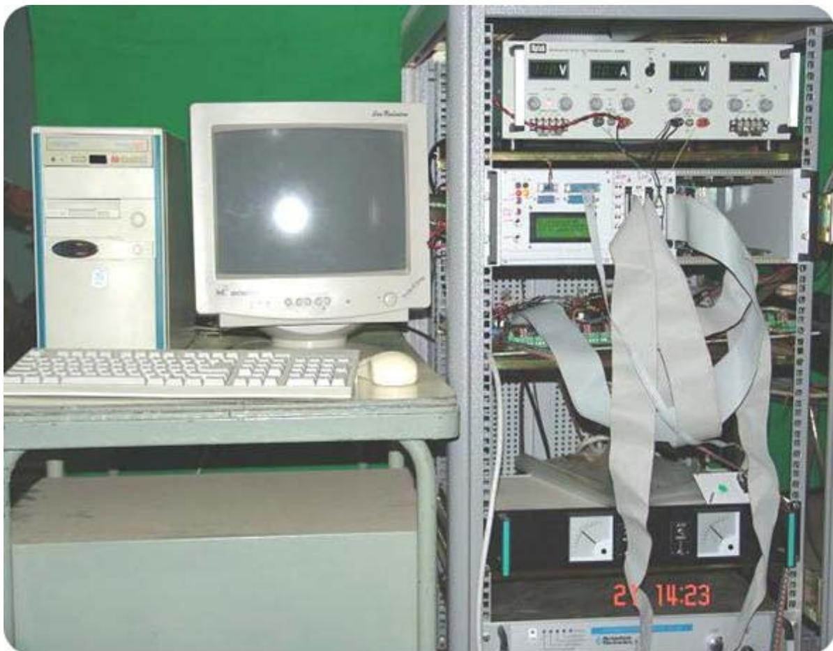
Fig. 13 : Computer control of Microwave Power Generator
