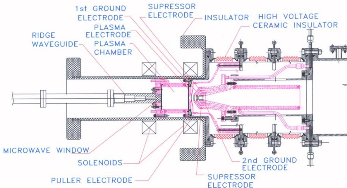
**Fig. 5 Schematic of the 50 keV, 50 mA ECR Proton Ion Source**
