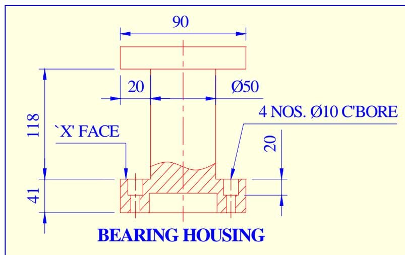
Fig.1: Schematic drawing of Bearing Housing
