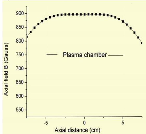
Fig. 15: Magnetic field profile for the ECR discharge
