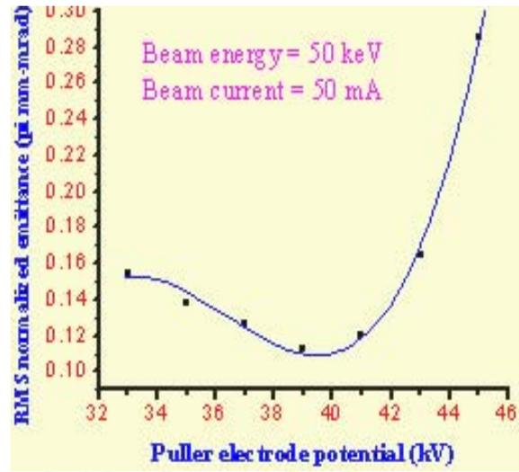
Fig. 9 Beam Emittance vs Puller Electrode Voltage
