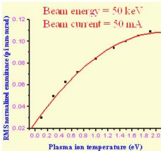
Fig. 8 Ion Source Emittance vs Plasma Ion Temperature
