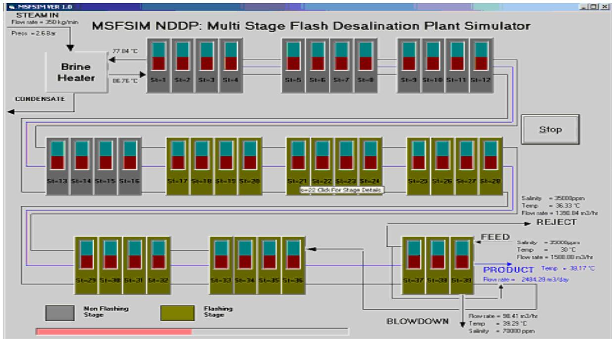
Fig. 2 Main form during Steady State simulation
