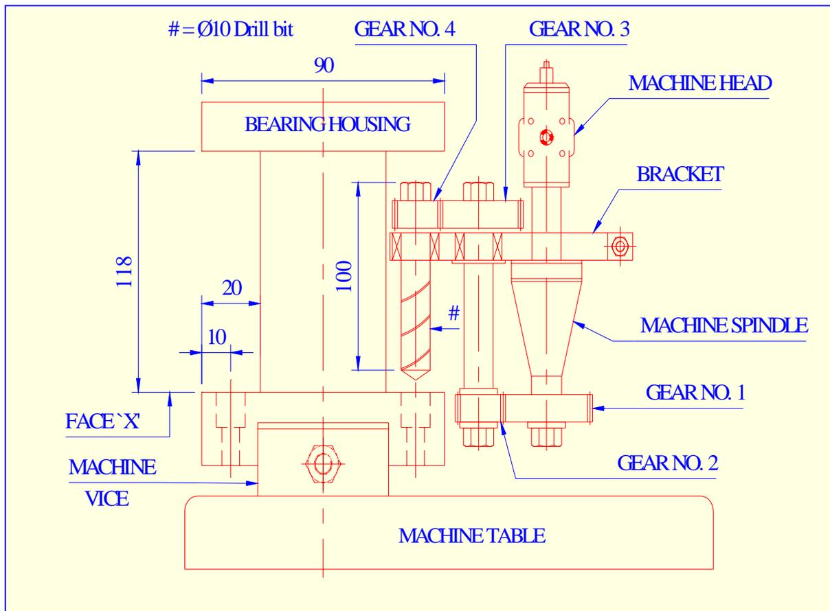
Fig.2 Schematic diagram of Counter Boring Attachment
