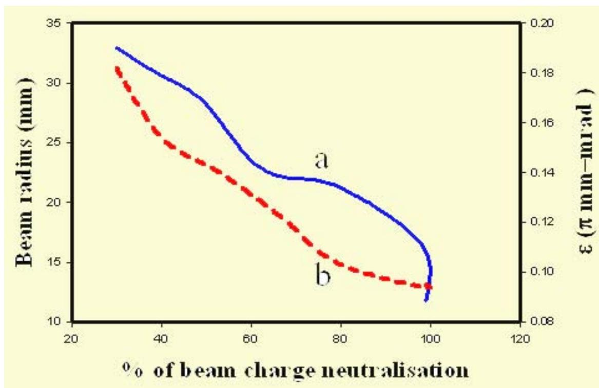
Fig. 10 Beam radius and beam emittance as a function of beam charge neutralisation
