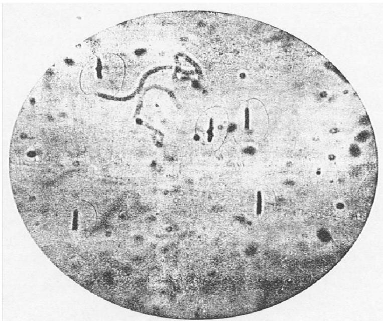
Fig. 3 Oriented fission tracks in Lexan from 60MeV helium ion induced fission of  $^{159}\text{Tb}$
