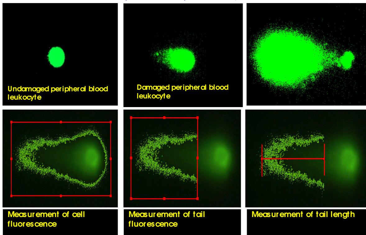
Fig. 4: Comets from control and proton irradiated cells and steps involved in measurements of comet characteristics using the software SCGE-PRO
