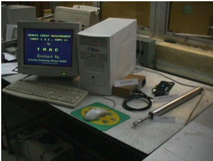
The software, which was developed in C language, was modified such that it takes care of different types of temperature correction factors to be applied on measured creep value for different combinations of pressure tube material and geometrical layout. It was also made compatible to ADC-528.
