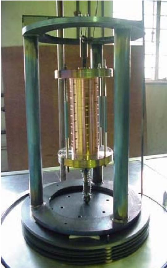
Fig. 4 : Holding fixture along with the 9 cells assembly
