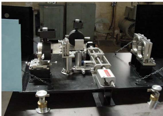
*Fig. 1. Layout of grating and mirror mounts*
