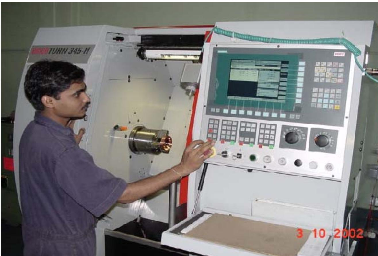
*Fig. 1 : R.F. Cavity being machined on a CNC precision lathe*
