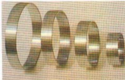
Ni-Ti shape memory alloy heat shrinkable sleeves
