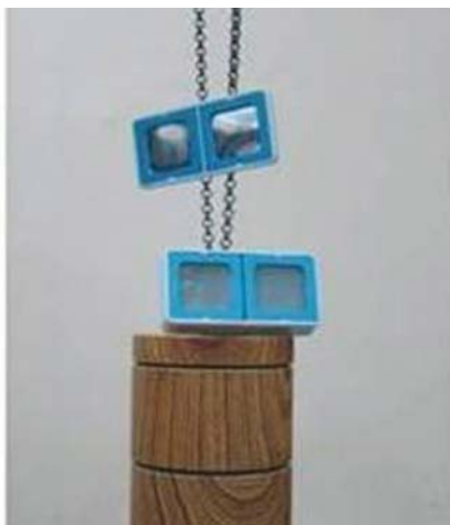
Fig.1: Detectors used for measurement of ^{220}\text{Rn} and ^{222}\text{Rn} gas and progeny concentrations
