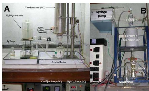
Fig. 1: Experimental set-up in quartz to carry out sulfuric acid decomposition (A) granular catalyst (20 g) and (B) powder catalyst (0.2 g)
