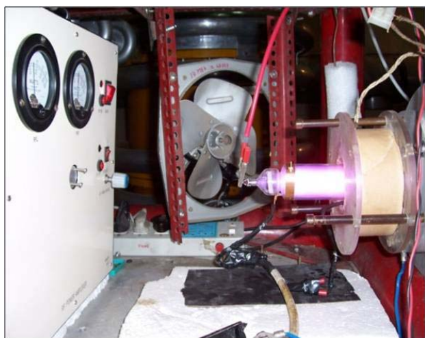
Fig.5: RF source with deuterium plasma
