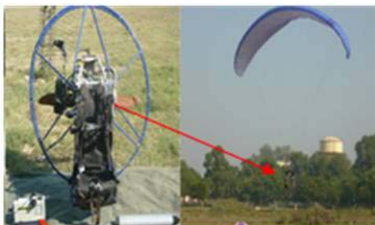
Fig.4:'Para Motor' based aerial trials using CARMS –for the assessment of ground level contamination and search of 'orphan sources'
