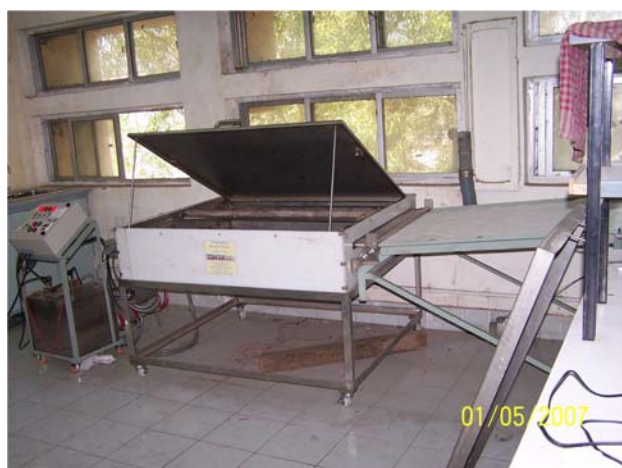
Fig. 5: Pilot scale Radiation Grafting Reactor system
