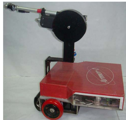
Fig.1: ARMER-I, Mobile robot with telescopic arm for monitoring radiation
