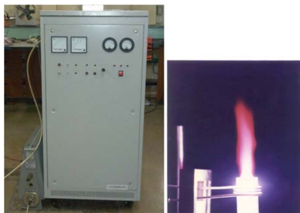
Fig. 6: RF generator: 27.12 MHz, 2 kW and (RF) argon plasma
