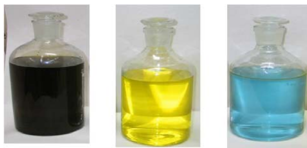
Fig. 4: The recovered plutonium and uranium from the analytical waste; (a) Waste, (b) U(VI), and (c) Pu(III) solutions
