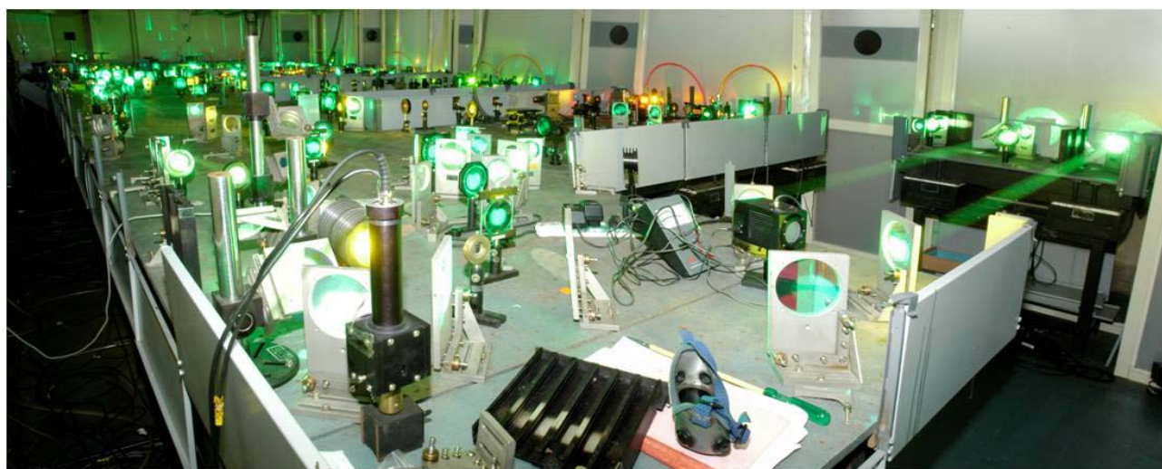
Fig. 3: High average power CVL pumped DL systems at our departmental facility during continuous round the clock operation
