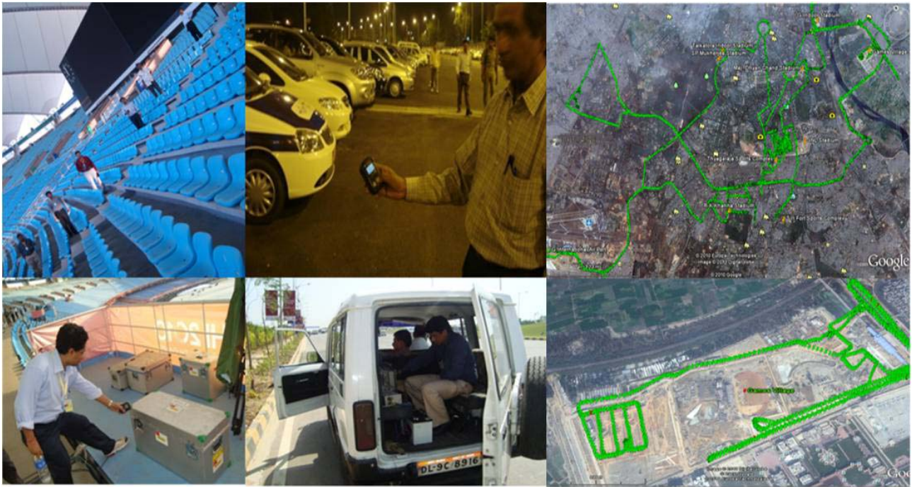
Fig.9: Ensuring 'Radiological Security and Safety' during Commonwealth Games (CWG-2010) through mobile radiation mapping (radiation level with positional coordinates and route followed) using AGSS and CARMs and screening of CWG stadia
