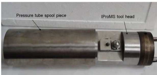
Fig. 5: IProMS tool head being inserted inside a heat treated spool piece of pressure tube
