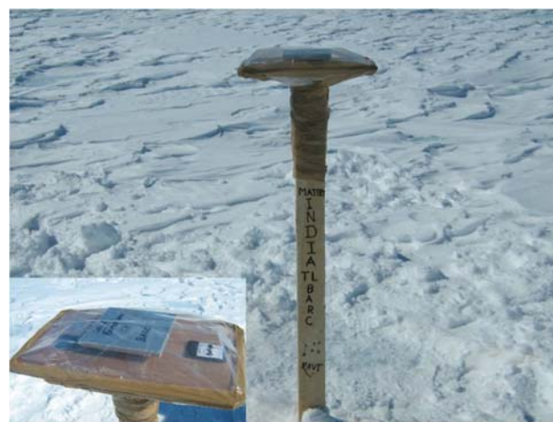
Fig.1: Photograph of TLD and CR-39 dosimeters deployed at Antarctica at a height of 1 m from the surface with a closer view on the left side.
