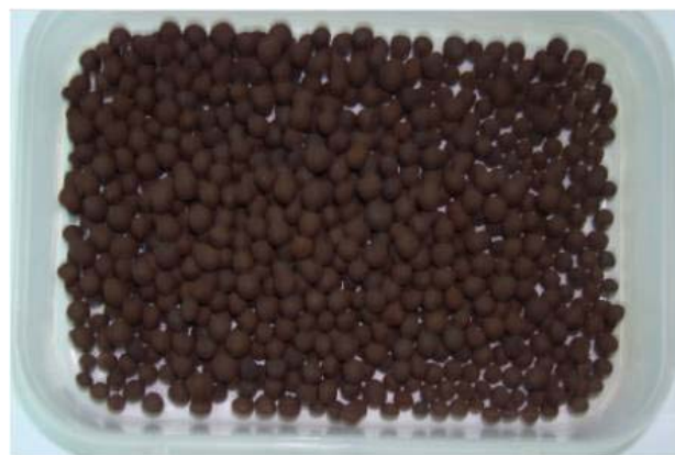
Fig. 2: Iron oxide based catalyst (Spherical granules, ~ 4-6 mm size)
