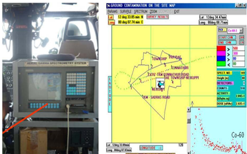
Fig.1: (a) AGSS installed in a Helicopter for aerial radiation mapping above 'simulated contamination' using combination of radioisotopes on ground. (b)AGSS screen display during an Aerial Survey above 'Simulated Radioactive Contamination on Ground' - spectrum showing Co-60 detected along with location displayed.
