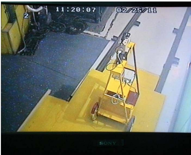
Fig.5: Mobile robot carrying Gamma/ Neutron survey meter inside K-130, cyclotron at VECC, Kolkata
