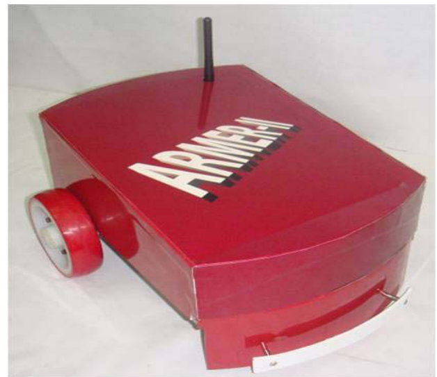
Fig.3: ARMER-II, Mobile robot for searching radioactive sources
