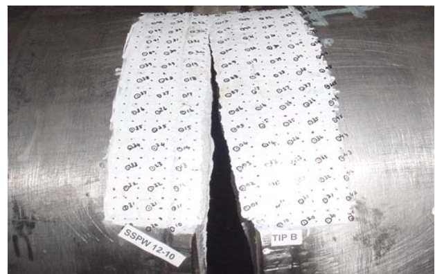
Fig. 8: Crack Growth in Pipe Weld of 168 mm OD
