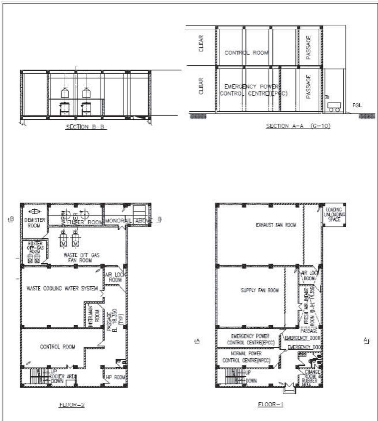
Fig. 2: General Arrangement of AWTF Annexe Building.
