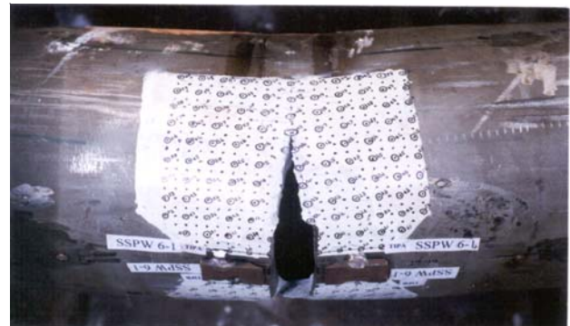
Fig. 7: Crack Growth in Pipe Base of 168 mm OD
