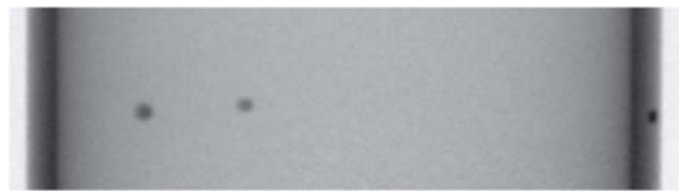
Fig. 2: Radiograph of zircaloy containing hydrogen blister
