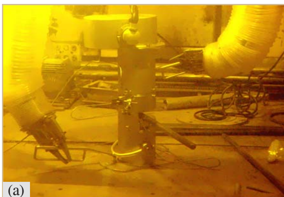
Fig. 3 : a) Remotely operated puncture chamber inside the hot cell and b) Pressure measuring part in the operating area outside the hot cells
