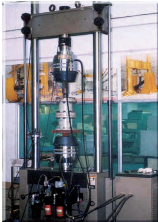
Fig. 16: Test carried out on Lead Extrusion Damper
