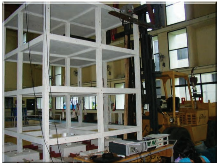
Fig. 42: Model structure ready for testing on tri-axial shake table
