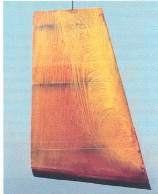
Fig. 15: Flow visualization at the partition plate of moderator inlet diffuser by tracer paint
