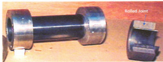
Fig. 2: Zero clearance pressure tube rolled joint spool and a sectioned joint
