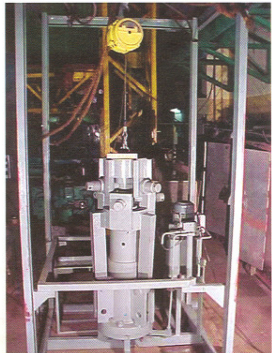
Fig. 6: Pull Out Test Facility
