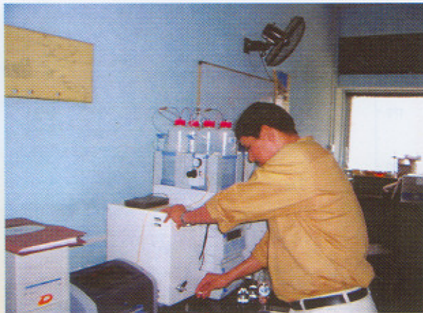
Fig. 5 : Dionex with gradient pump ion chromatographic system GD50 and electrochemical detector ED50, PDA UV-VIS detector UVD 340, sample changer AS 50 Column for anions, cations and transition elements and lanthanides and chromeoleon ion chromatography software
