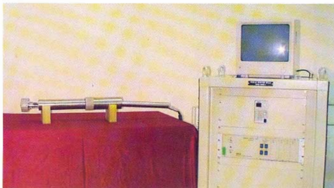
Fig. 1 Miniature Underwater Radiation Resistant CCTV Camera System
