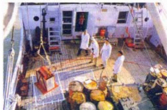
Plate 2 Mixing of ^{46}\text{Sc} tracer in the injection apparatus
