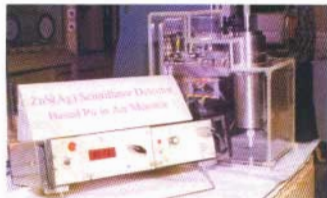
Fig. 1 ZnS(Ag) scintillator detector based Pu-in-Air monitor
